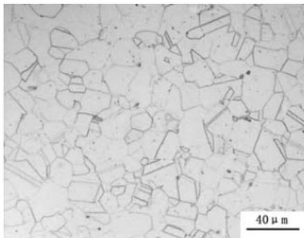
1 Micrograph of as received GH4169 superalloy before isothermal compression
