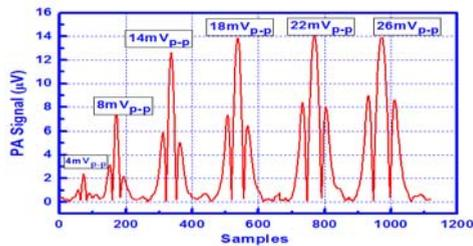
Fig.3.  $C_2H_2$  transitions near 1530.371 with modulation depths varying from 4mVp-p to 26mVp-p
