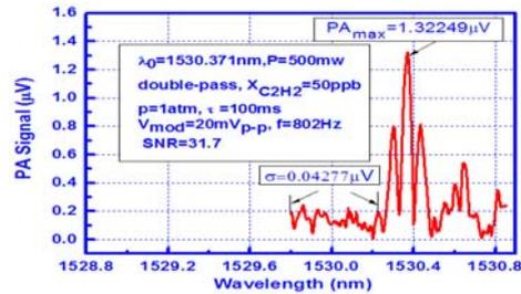
Fig.48. Measured 2f spectra of 50ppb flowing  $C_2H_2$  in synthetic air at optimum conditions
