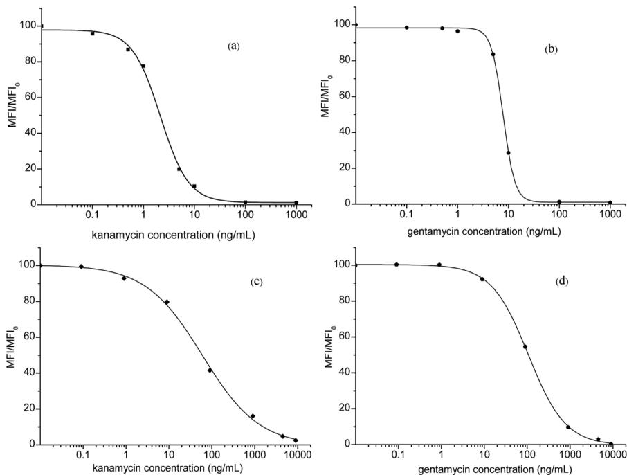
Figure 3. Standard curves of kanamycin and gentamycin in PBS and in milk extract. (a) and (b) were obtained simultaneously in PBS; (c) and (d) were obtained simultaneously in milk extract.
