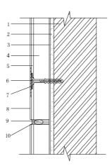
1 wall structure, 2 cement mortar lever, 3 mortar glue, 4 composite board, 5 fibre reinforced layer 6 bolt, 7 reinforced net, 8 face brick, 9 Polyethylene foam, 10 sealant
