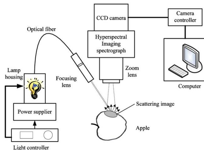
Fig. 1. Schematic of the hyperspectral imaging system for acquiring scattering images from apples.
