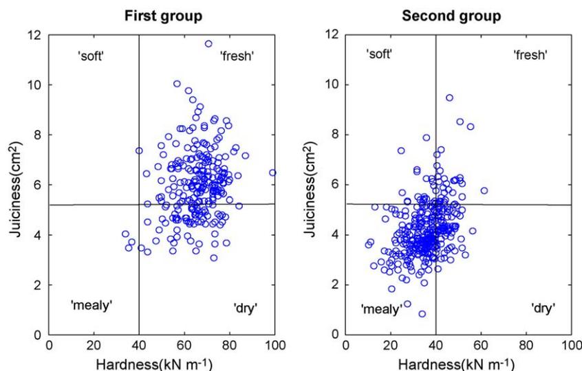
**Fig. 3.** Classification of apple samples based on the destructive confined compression tests. Apples for the first group were kept in cold storage at  $4^\circ\text{C}$  and those in the second group were kept at room temperature ( $20^\circ\text{C}$ ) with 95% relative humidity.
