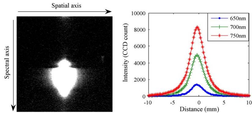
Fig. 2. Hyperspectral scattering image of an apple (left), and raw spatial scattering profiles at three wavelengths (right).
