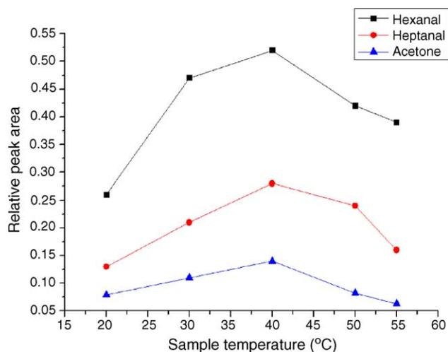
Fig. 1. Influence of sample temperature on the relative peak area of acetone, hexanal and heptanal oximes. Extraction conditions: drop volume, 1  $\mu$ l; extraction time of 4 min; stirring rate, 5000 rpm.
