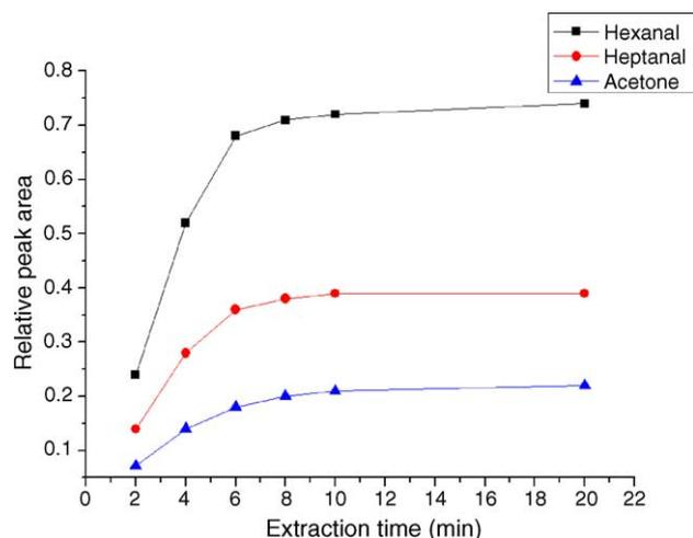
Fig. 2. Influence of extraction time on the relative peak area of acetone, hexanal and heptanal oximes. Extraction conditions: sample temperature, 40 °C; drop volume, 1  $\mu$ l; stirring rate, 5000 rpm.
