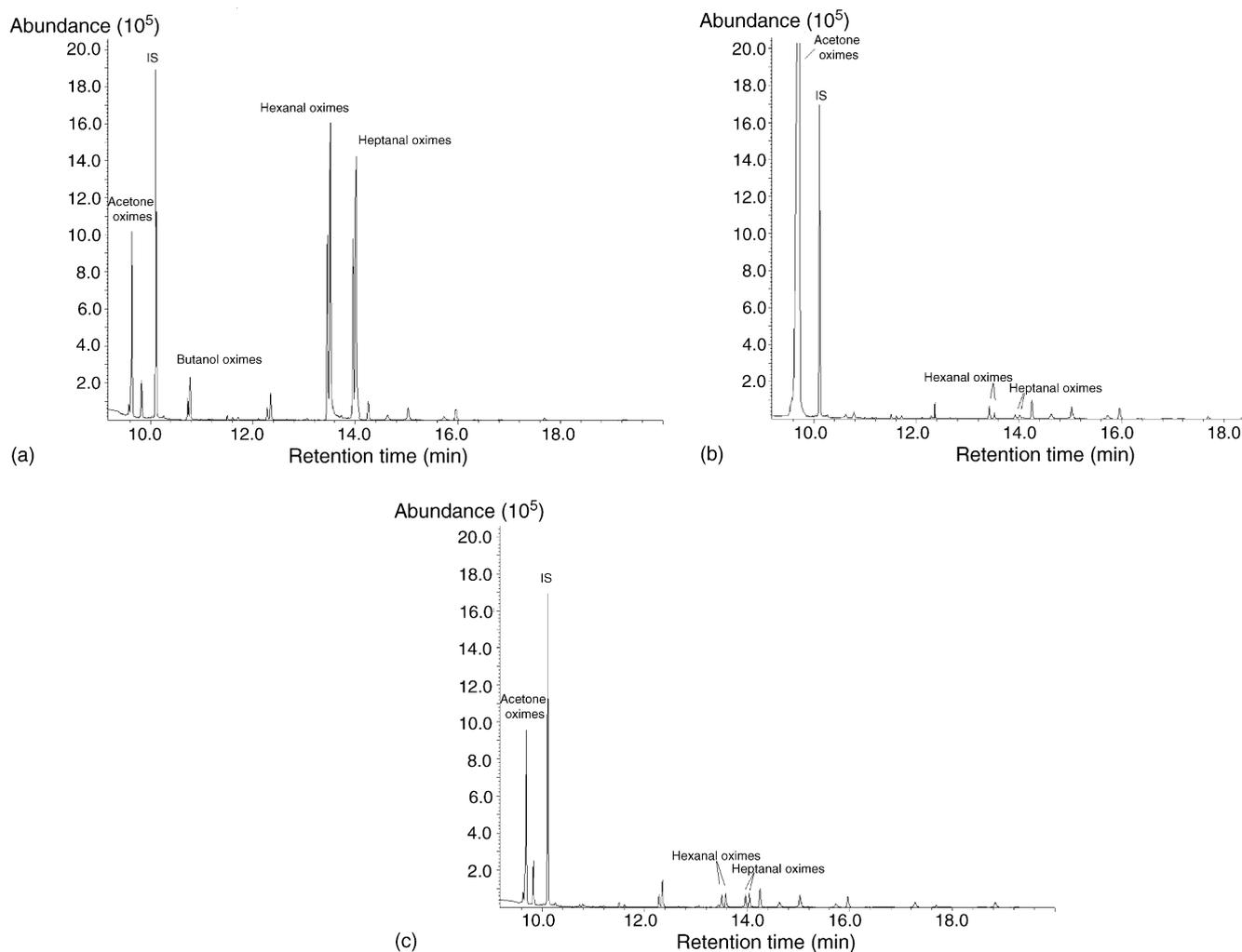
Fig. 3. The total ion chromatograms of a lung-cancer blood: (a) a diabetic blood; (b) and a control blood; (c) by PFBHA derivatization followed by HS-SDME and GC-MS.
