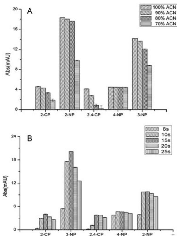
**Figure 1.** Effects of ACN in water (A) and desorption volume (B) on the desorption of nitrophenols for the in-line concentrator. Standard solutions of  $200 \text{ ng mL}^{-1}$  at pH 7.5 were used. Extraction and CE conditions are described in Section 2.5.
