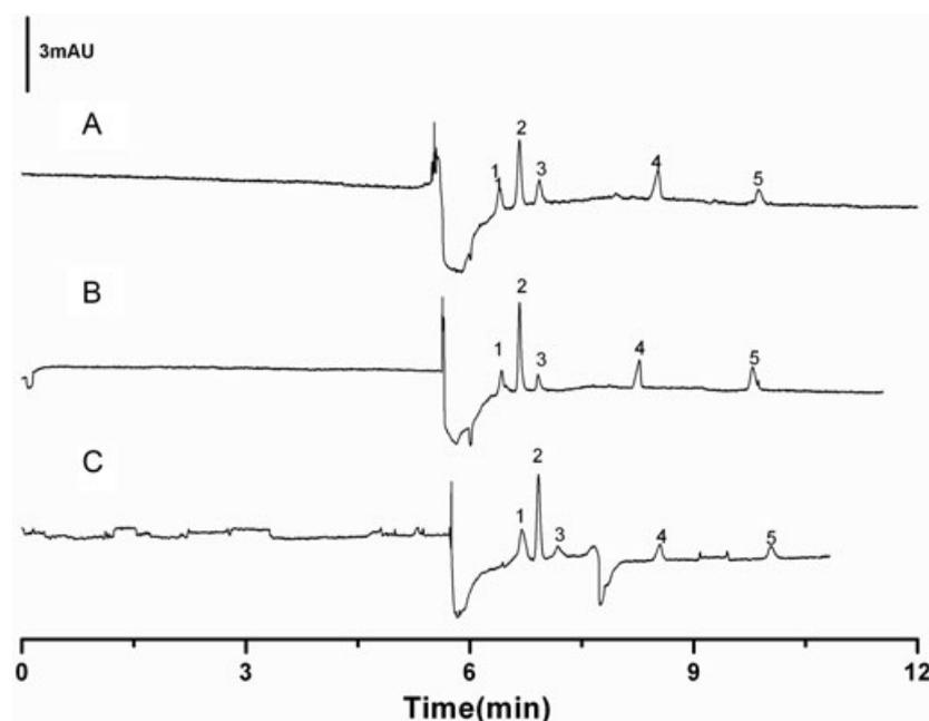
**Figure 4.** Electropherograms of separating phenols by in-line polymeric SPE-CE for real water samples (A) snow water (B) tap water (C) Yangtze River water spiked with 20 ng mL<sup>-1</sup> of each phenol. Peak identification: (1) 2-CP; (2) 3-NP; (3) 2,4-CP; (4) 4-NP; (5) 2-NP. Other conditions are the same as in Fig. 1.
