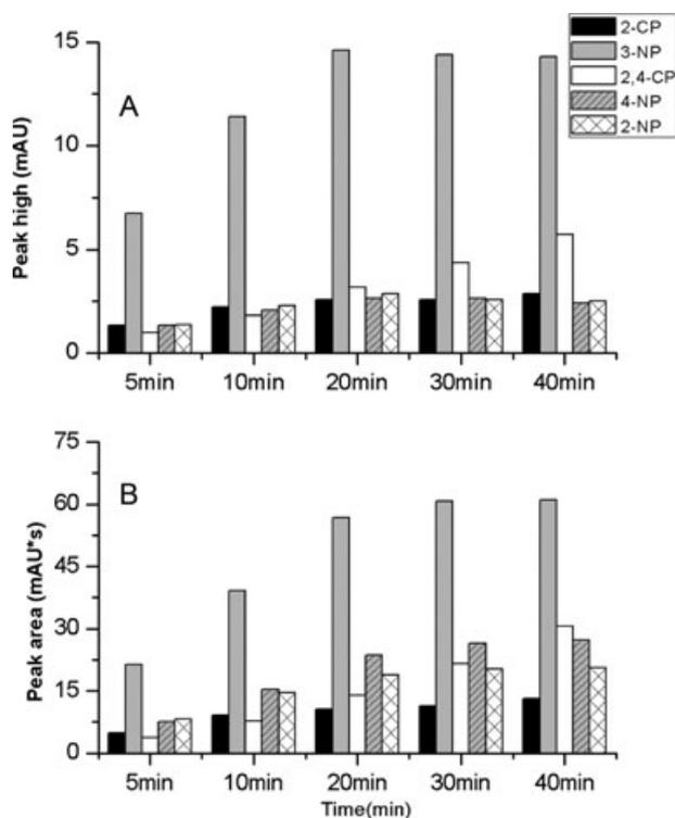
**Figure 2.** Effects of sample loading time on individual peak heights (A) and individual peak areas (B) of five phenols with in-line concentration. Other conditions are the same as in Fig. 1.
