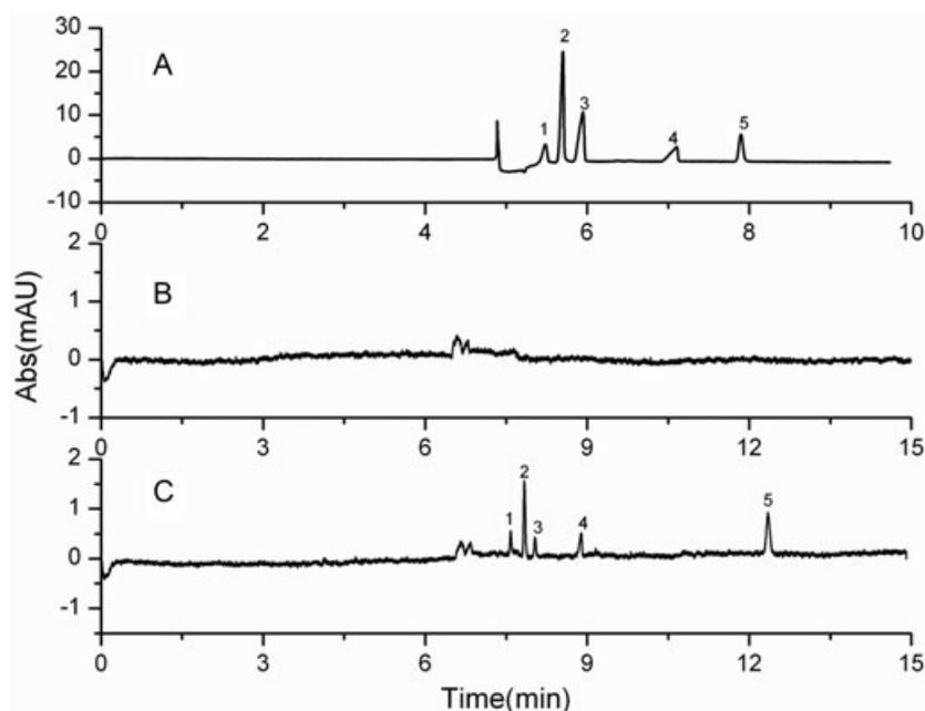
**Figure 3.** Electropherograms of separating phenols (A) by polymeric SPE-CE at sample concentration of 500 ng mL<sup>-1</sup> (B) by CE at sample concentration of 500 ng mL<sup>-1</sup> (C) by CE at sample concentration of 20 μg mL<sup>-1</sup>. Peak identification: (1) 2-CP; (2) 3-NP; (3) 2,4-CP; (4) 4-NP; (5) 2-NP. Other conditions are the same as in Fig. 1.
