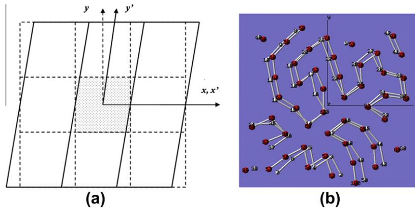
Fig. 7. Deformation of uniform shear along the  $x$ -axis.
