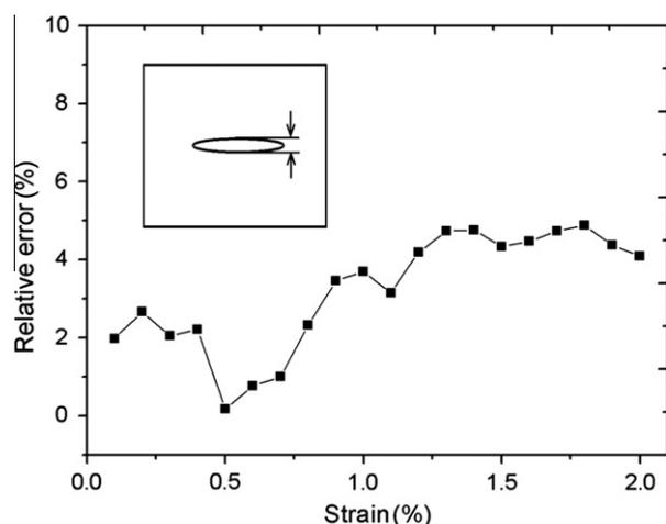
**Fig. 12.** The relative error of crack opening displacement vs. the applied strain.
