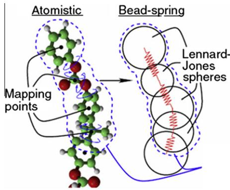
Fig. 1. Schematic of coarse grain method (Ref. [9]).
