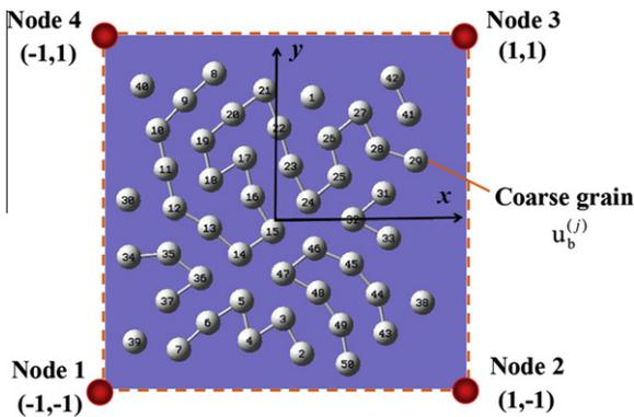
Fig. 4. Geometry of a four-node element.
