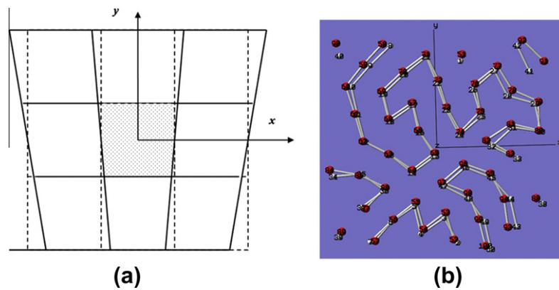
Fig. 8. Deformation of non-uniform stretch along the  $x$ -axis.
