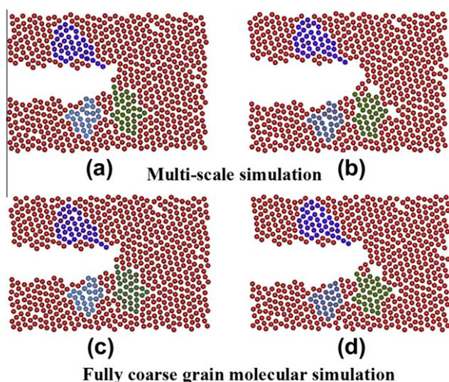
**Fig. 11.** Deformation around crack tip for two different loadings: (a) and (b) simulated by the multi-scale method, (c) and (d) modeled by the fully coarse grain method.
