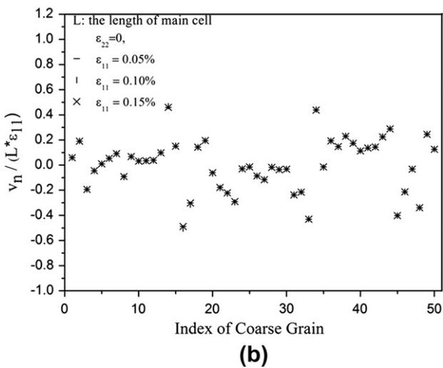
Fig. 6. Displacements of coarse grains along the x-axis (a) and the y-axis (b).
