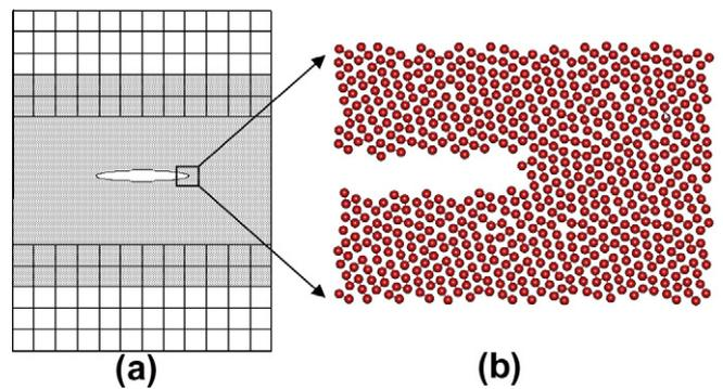
Fig. 10. (a) Multi-scale simulation of polymer fracture, (b) the initial coarse grain configuration near crack tip.
