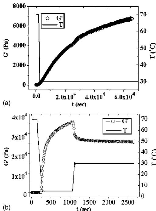
FIG. 4. Rheological tests of 2% w/v agarose systems. (a) Elastic modulus evolution curve for the gel formed by directly quenching the gelling system to 30 °C.  $G'_\infty \approx 8700$  Pa is obtained by data extrapolation using the plot of  $G'$  vs  $1/t$  (not shown). (b) Elastic modulus evolution curve for the gel formed by first quenching the system to 5 °C and then heating the system back to 30 °C.
