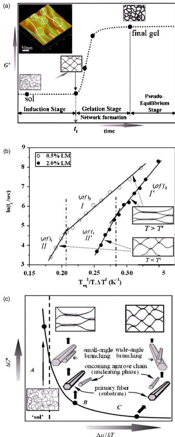
FIG. 2. (Color online) (a) Schematic illustration of agarose gelation process. Inset: Atomic force microscopy micrograph image of 2% w/v agarose gel network formed under 22 °C (network junctions are highlighted by dotted circles). (b) The plot of  $\ln(t_i)$  vs  $T_{eq}^2/T\Delta T^2$ . The solid lines are obtained by linear fitting. (c) Illustration of gel network formation through nucleation. As for  $\Delta\mu/kT$  and  $\Delta G^*$ , see Eq. (2).
