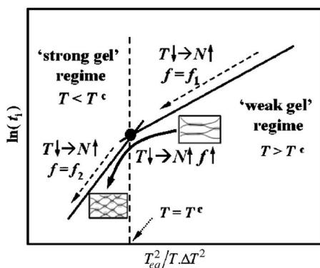
FIG. 3. Illustration of the protocol used to fabricate significantly enhanced gel networks.  $T$ , the final setting temperature;  $T^c$ , the critical final setting temperature;  $N$ , the junction number of the hydrogel network; and  $f$ , the factors describing the structural correlation between the primary fiber (substrate) and the oncoming agarose chain (nucleating phase),  $f_2 > f_1$ .
