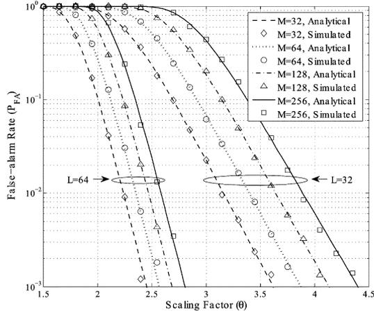
Fig. 1. Relationship between  $P_{FA}$  and  $\theta$  over a few combinations of  $L$  and  $M$ . Simulations are conducted with SNR assumed to be  $-10$  dB.
