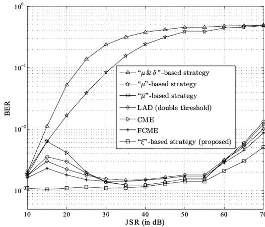
Fig. 3. BER versus JSR.  $E_b/N_0 = 8$  dB,  $\alpha = 25\%$ . Simulations repeated for  $5 \times 10^5$  QPSK symbols.
