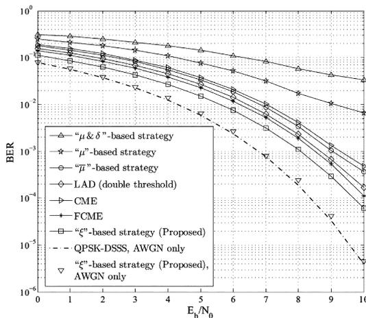
Fig. 4. BER versus  $E_b/N_0$ .  $\alpha = 25\%$ , JSR = 20 dB (if not otherwise noted). Simulations repeated for  $5 \times 10^7$  QPSK symbols.
