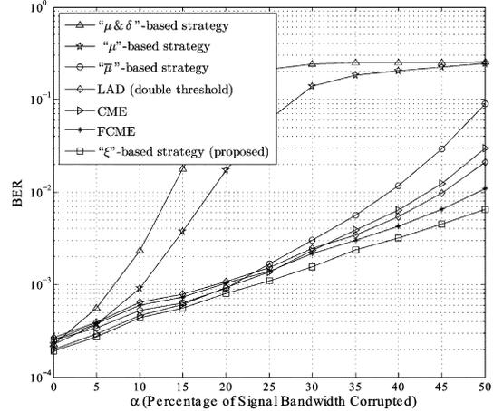
Fig. 2. BER versus  $\alpha$ .  $E_b/N_0 = 8$  dB, JSR = 30 dB. Simulations repeated for  $5 \times 10^5$  QPSK symbols.  $\alpha = 0$  denotes sinusoid jammer.
