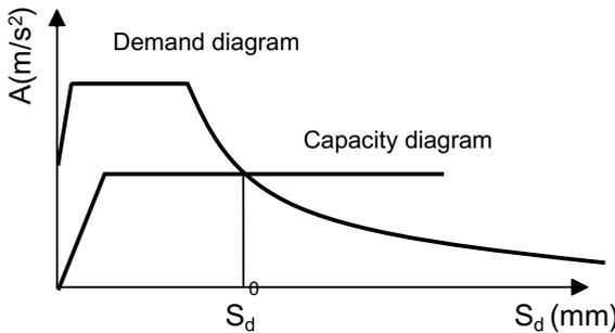
Fig. 1. Capacity–demand diagram method.
