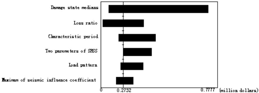
Fig. 14. Tornado diagram analysis of earthquake loss.
