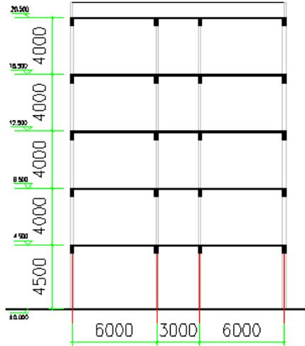
Fig. 6. Elevation view of the hotel (mm).
