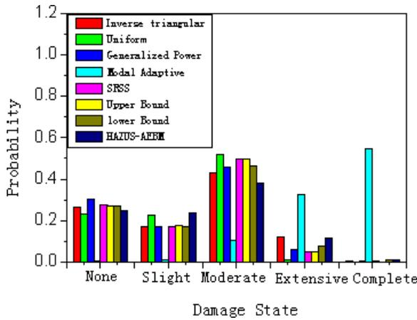
Fig. 8. Damage probability of lower bound of spectral displacement.
