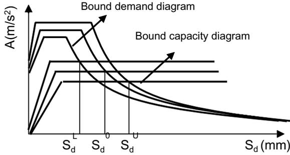
Fig. 2. Bound capacity–demand diagram method.
