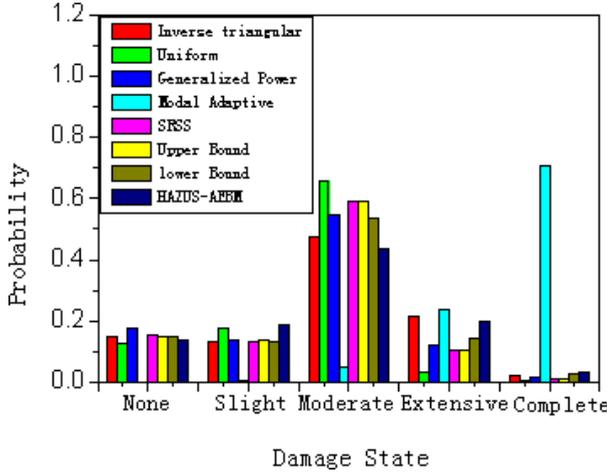
Fig. 9. Damage probability of medians of spectral displacement.
