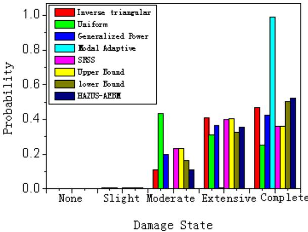
Fig. 10. Damage probability of upper bound of spectral displacement.
