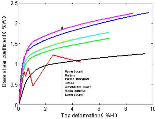
Fig. 7. Pushover curves for the example structure under five load patterns.
