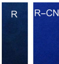
Figure 8. (Colour online) Photographs of R of test papers of only R and after immersion into DMSO–H 2 O (8:2, v/v, 0.01 M HEPES, pH 7.21) solution with CN − under irradiation at 365 nm.
