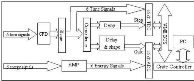
Figure 1. block diagram of data acquisition system
