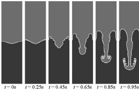
Fig.7 The evolution of Rayleigh-Taylor instability with time using FCT-VOF method
