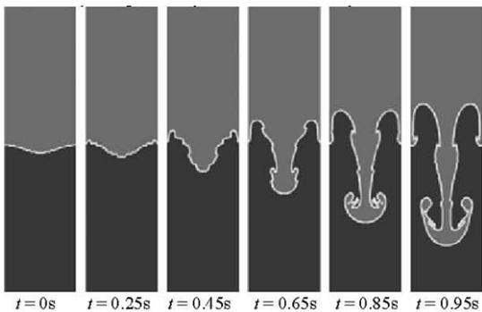
Fig.8 The evolution of Rayleigh-Taylor instability with time using SLA scheme
