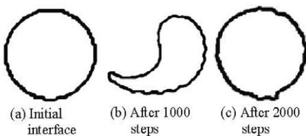
Fig.4 The simulation results with the FCT-VOF method
