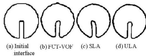
Fig.3 The slotted circle simulated after a rotation cycle
