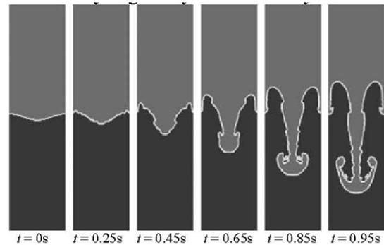
Fig.9 The evolution of Rayleigh-Taylor instability with time using ULA scheme
