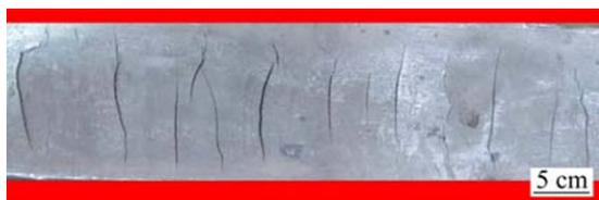
Fig. 6 Strip at casting temperature of 680 °C
