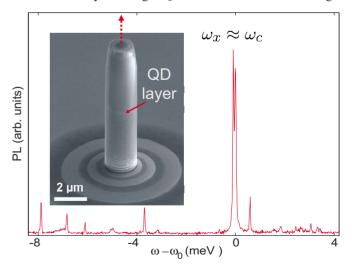
FIG. 1. (Color online) Typical broadband PL spectrum that is emitted when a target exciton is closely resonant with the cavity mode (near  $\omega_0$ =1331.355 meV); away from the target exciton, there are a series of other exciton levels that can also couple, offresonantly, to the cavity mode. The SEM image shows our micropillar cavity and the QD layer. The emitted photons from the QDs are detected through vertical emission.
