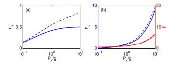
FIG. 4. (Color online) (a) Mean exciton number versus  $P_x$  (with  $P_c=1.6P_x$ , as before): exciton pump thermal-bath model (solid) and laser model (dashed); both cases include stimulated emission. (b) Corresponding mean photon number (left axis: blue) and Fano factor *F* (right axis: red).
