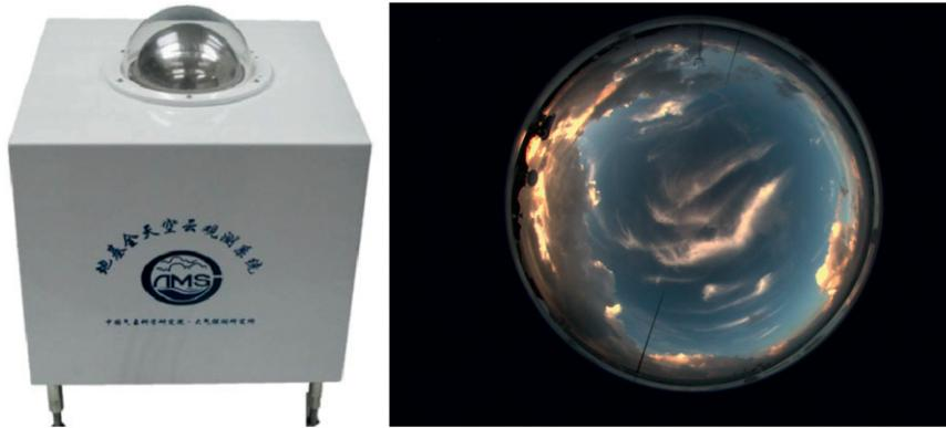
FIG. 1. Ground-based TCI: (left) TCI device and (right) an example of TCI image obtained at 0625 local time (LT) 30 Jun 2010 in Yangjiang, China.
