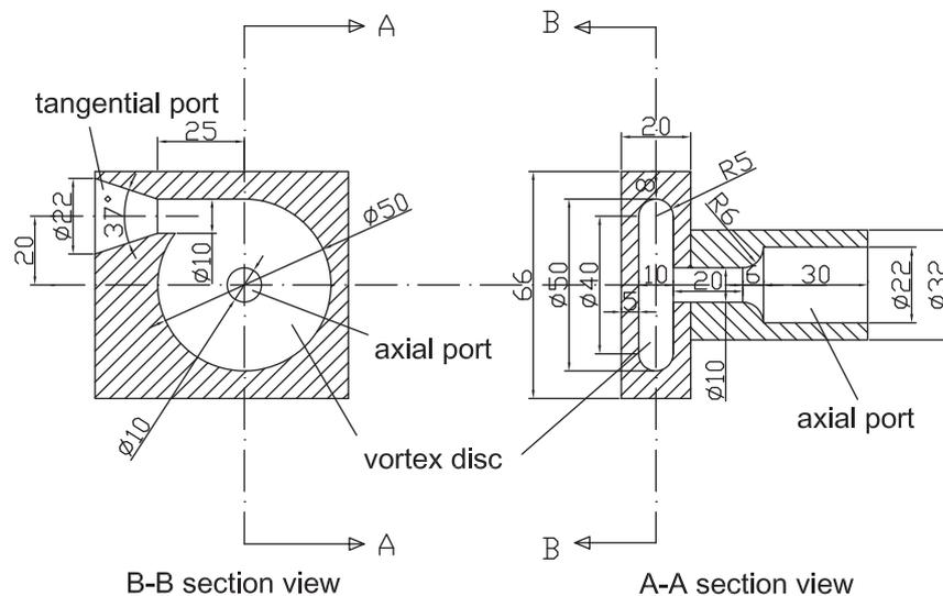
Fig. 10. Configuration of the vortex diode used to inhibit the leakage of compressed gas during the compression phase.
