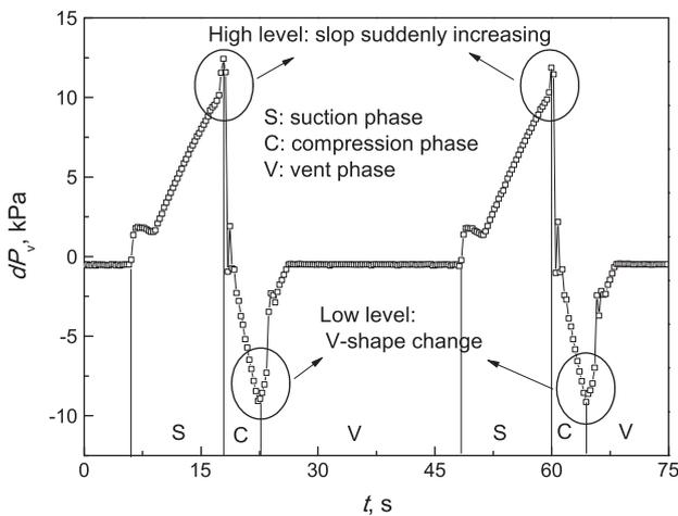
Fig. 8. Pressure difference data  $dP_v$  acquired in real time (mixing nozzle B;  $d_1$ , 4 mm;  $d_2$ , 6 mm;  $D$ , 17.25 mm;  $H_b$ , 10 cm;  $H_l$ , 120 cm;  $H_v$ , 5.0 cm).
