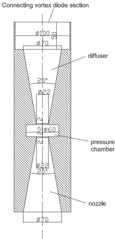
Fig. 6. Venturi tube for maximum-level detection in the gas ballast.
