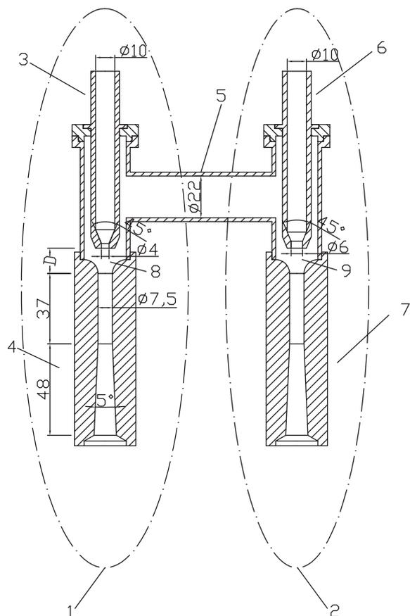
Fig. 3. Geometric configuration of JPP.
