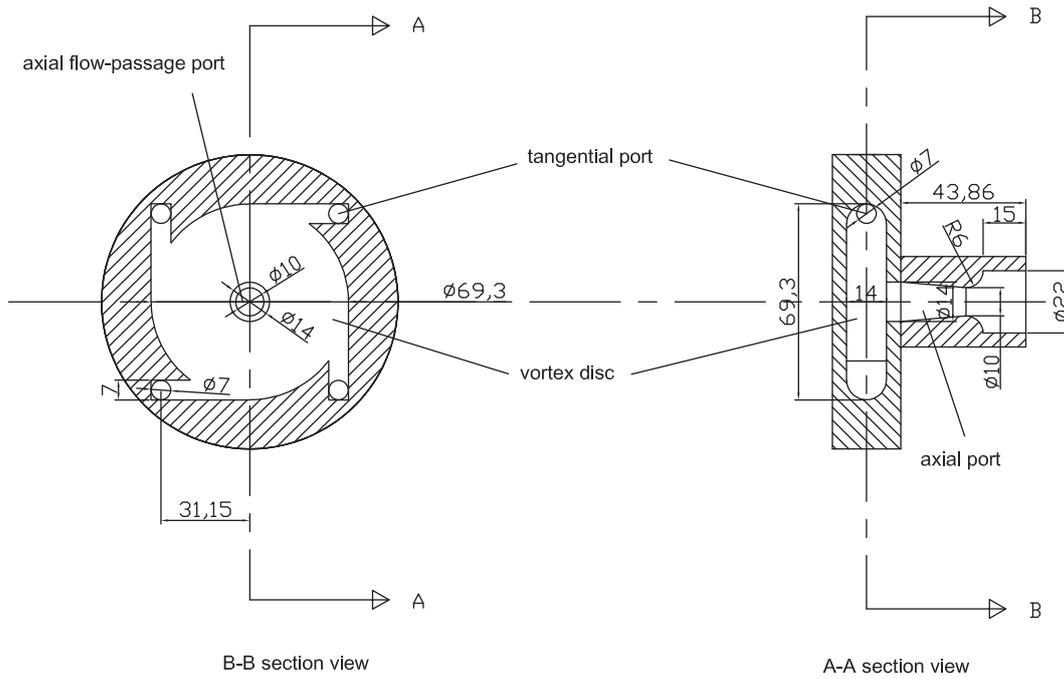
Fig. 7. Vortex diode used to prevent fluid from overflowing out of the gas ballast.
