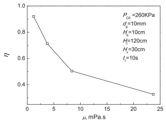
Fig. 18. Effects of liquid phase viscosity on the average mixing index.
