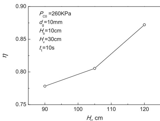
Fig. 20. Effects of maximum fluid level in the gas ballast on the average mixing index.
