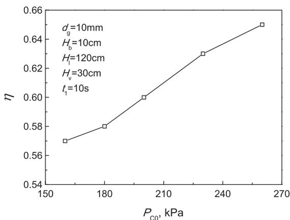
Fig. 15. Effects of static pressure of the compressed air on the average mixing index.
