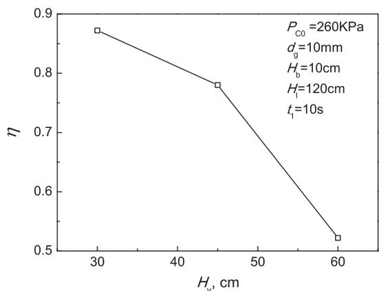
Fig. 19. Effects of fluid level in the storage tank on the average mixing index.
