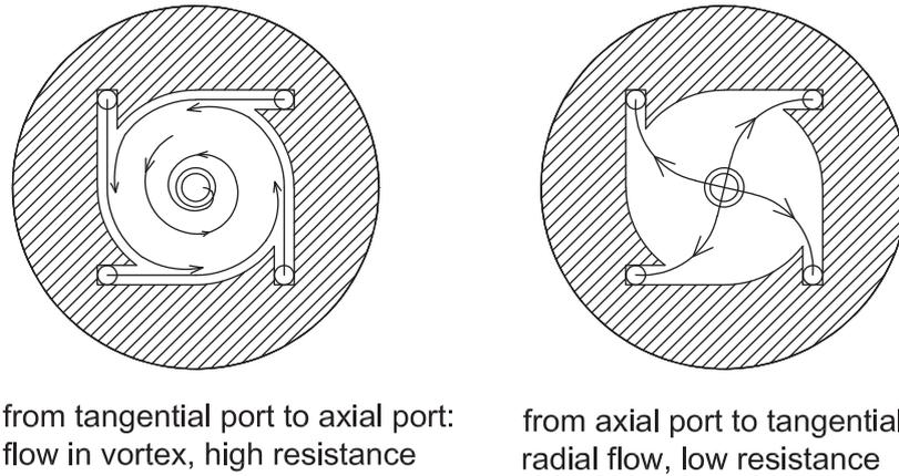
Fig. 9. Working principle of vortex diode.
