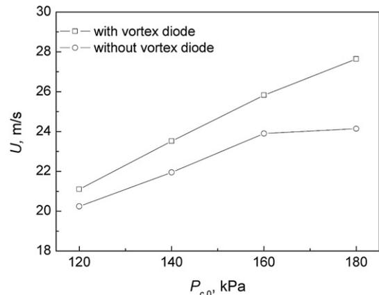
Fig. 13. Effects of vortex diode on mixing jet flow velocity (mixing nozzle B,  $d_1$ , 4 mm;  $d_2$ , 6 mm;  $D$ , 17.25 mm;  $H_b$ , 10 cm;  $H_1$ , 120 cm;  $H_v$ , 50 cm).
