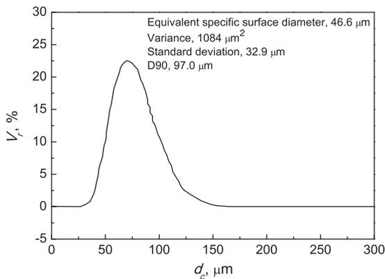
Fig. 5. Particle size distribution of quartz sand.
