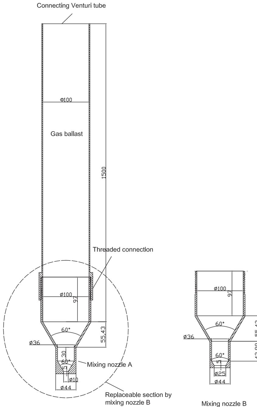
Fig. 2. Geometric configuration of PJM.
