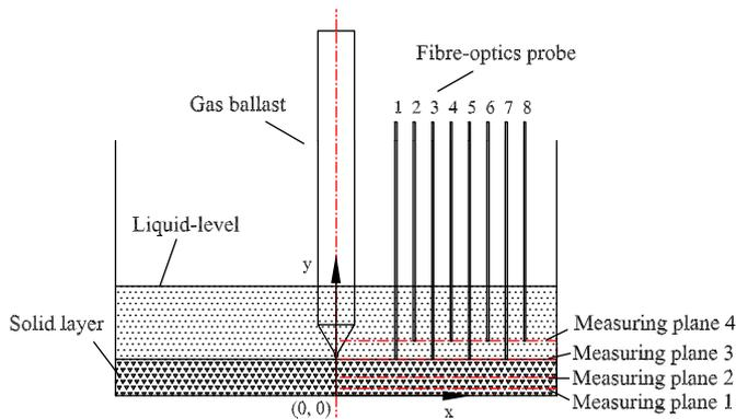
Fig. 14. Layout of fiber-optic probes in the storage tank.
