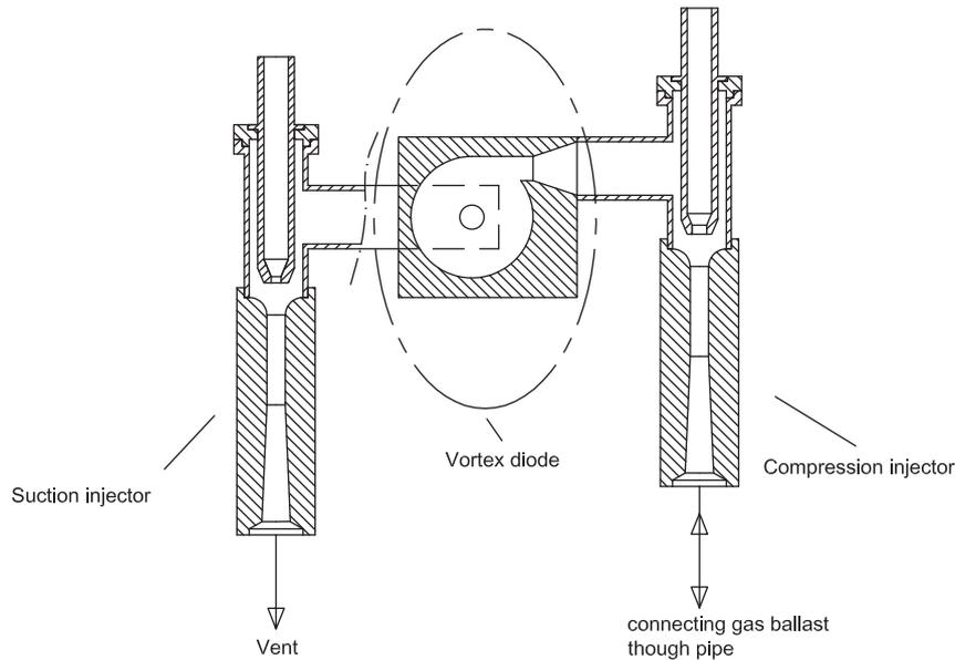
Fig. 11. Layout of JPP with a vortex diode.
