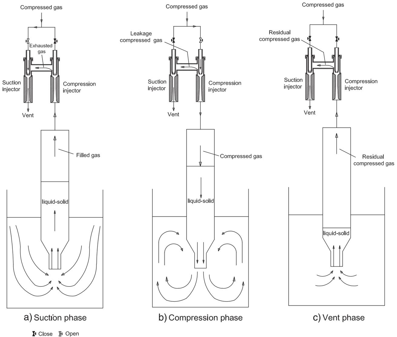
Fig. 4. Working processes of PJM.
