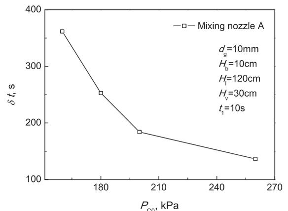
Fig. 17. Effects of static pressure of the compressed air on local stable mixing time.
