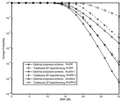
Fig. 5. Outage probability vs SNR for the proposed scheme and traditional ZF beamforming with different settings of relay antennas,  $M = 4$  and  $R_t = 5$  bit/s/Hz.
