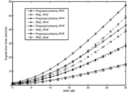
Fig. 2. Ergodic sum rate vs SNR for the proposed scheme and PNC.  $M = 2, 4, 6, 8$  and  $N = 2M - 1$ .
