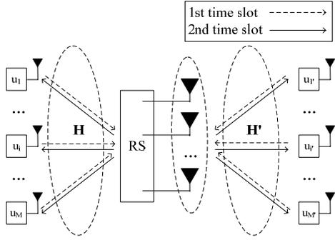
Fig. 1. Multi-pair two-way relay channels scenario for the proposed protocol.
