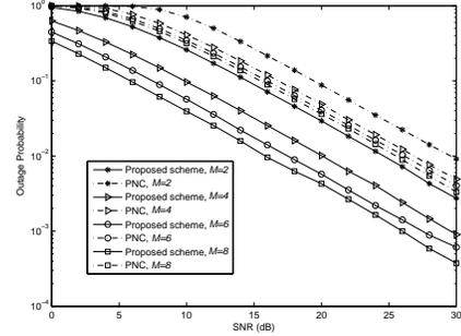
Fig. 3. Outage probability vs SNR for the proposed scheme and PNC.  $M = 2, 4, 6, 8$ ,  $N = 2M - 1$  and  $R_t = 2$  bit/s/Hz.
