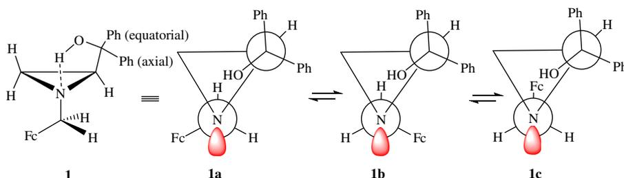
Figure 3. Three conformations about the N–C bond rotation for ligand **1**.
