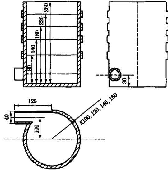
Fig. 6 Schematic of cylindrical swirling chamber
