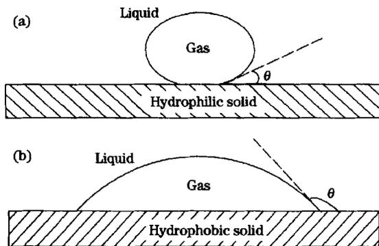
Fig. 1 Two statuses of three-phase configuration
