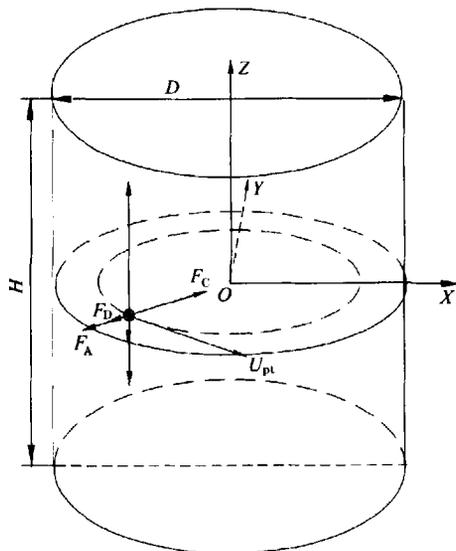
Fig. 4 Schematic of forces on an inclusion particle
