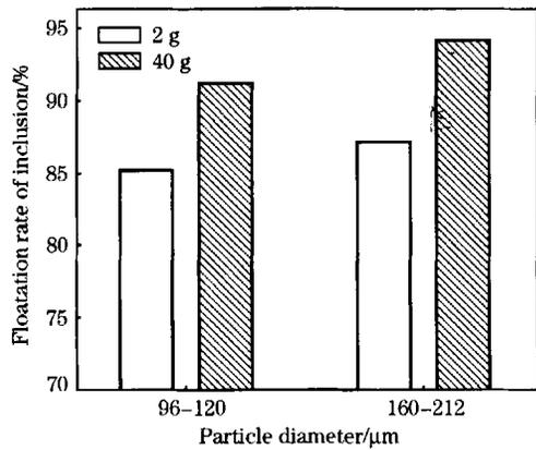
Fig. 7 Variation of inclusion floatation rate with particle size and quantity
