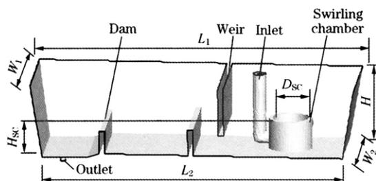
Fig. 5 Single strand swirling flow tundish configuration
