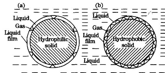
Fig. 2 Different particle surfaces adsorbed micro bubbles in liquid media
