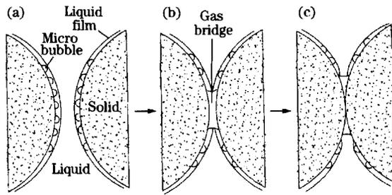
Fig. 3 Formation of gas bridge and rupture of liquid film between solid surfaces coated with micro bubbles
