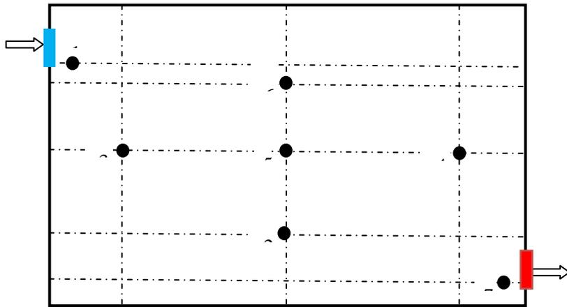
**Fig. 4.** Test points in the chamber (sectional view).
