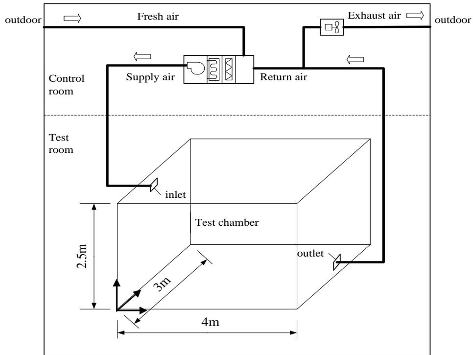
**Fig. 3.** System sketch of measurement.
