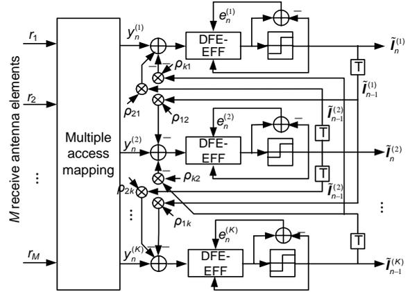
Fig. 3 Scheme of the MIMO MIC DFE-EFF multiuser detector
