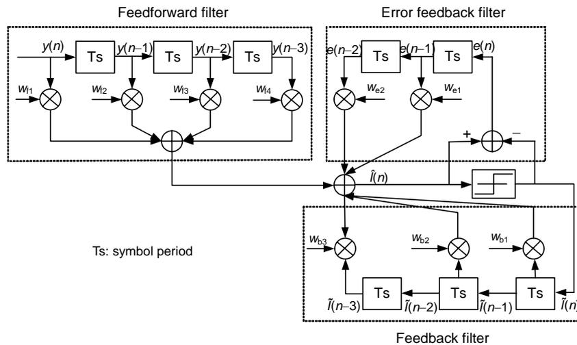
Fig. 2 Scheme of the decision feedback equalizer with error feedback filter (DFE-EFF) (Saif, 2003)
