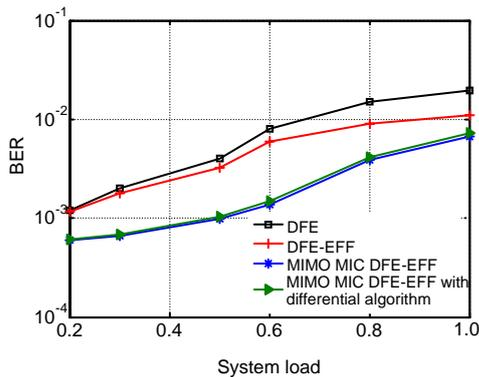
Fig. 8 System performance as a function of the system load ( $K/N_s$ ) at an SNR of 10 dB
