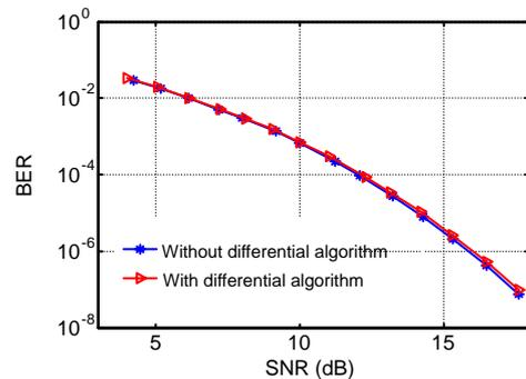
**Fig. 7 BER performance of multistage MIMO MIC DFE-EFF with and without the differential algorithm, for eight spread factors and three iterations**
