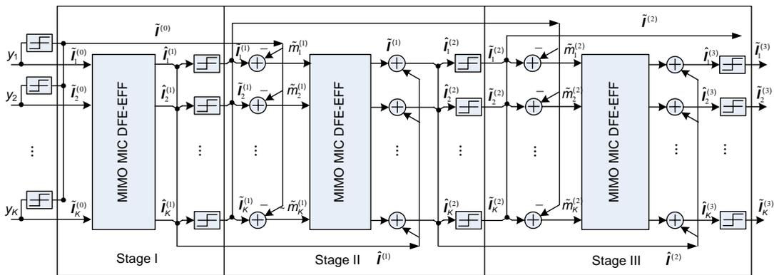
Fig. 4 Differential structure of a multistage MIC DFE-EFF detection system
