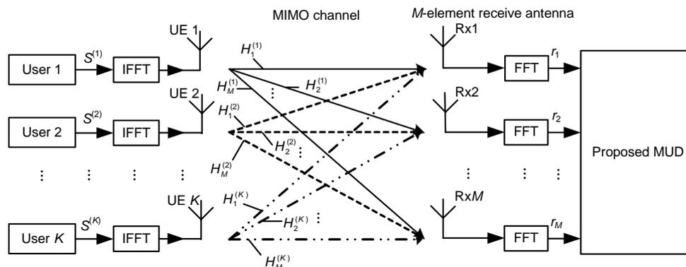
Fig. 1 Scheme of the uplink multiuser MIMO-OFDM system model (Hanzo and Keller, 2006) with the proposed multiuser detection (MUD)
