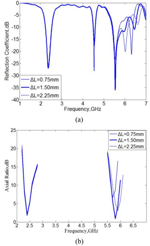
Fig. 8. Simulated (a) reflection coefficient and (b) axial ratio against frequency for various  $\Delta L$ .  $R = 14$  mm,  $d_p = 4$  mm,  $W_p = 3$  mm, and  $L1 = 8$  mm.
