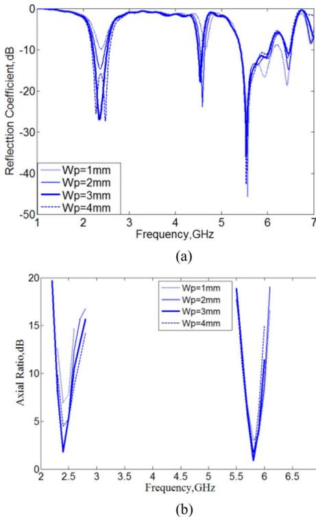
Fig. 7. Simulated (a) reflection coefficient and (b) axial ratio against frequency for various  $W_p$ .  $R = 14$  mm,  $d_p = 4$  mm,  $L1 = 8$  mm, and  $\Delta L = 1.5$  mm.
