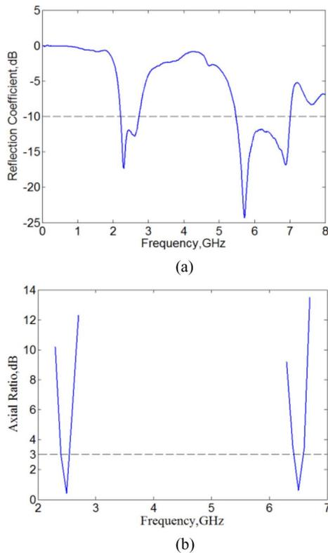
Fig. 9. Measured (a) reflection coefficient and (b) axial ratio for antenna prototype with  $\epsilon_r = 4.2$ ,  $h = 1.45$  mm;  $R = 14$  mm,  $d_p = 4$  mm,  $W_p = 4$  mm,  $L_1 = 8$  mm,  $\Delta L = 2$  mm,  $S_1 = S_2 = 1$  mm;  $W_t = 0.96$  mm,  $L_t = 18$  mm, and  $L_s = 0$  mm.
