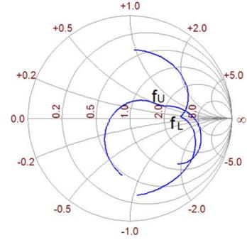
Fig. 2. Impedance seen at the edge of the ring slot of the antenna (without impedance transformer);  $L_s = 1$  mm,  $W_t = 2.8$  mm;  $f_L = 2.4$  GHz,  $f_U = 5.8$  GHz.
