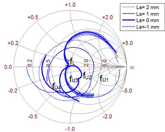
Fig. 5. Effect of various  $L_s$  on the input impedance of the antenna;  $W_t = 0.9$  mm,  $L_t = 18$  mm;  $f_L = 2.4$  GHz,  $f_{U1} = 5.7$  GHz,  $f_{U2} = 5.8$  GHz,  $f_{U3} = 5.8$  GHz, and  $f_{U4} = 5.9$  GHz.
