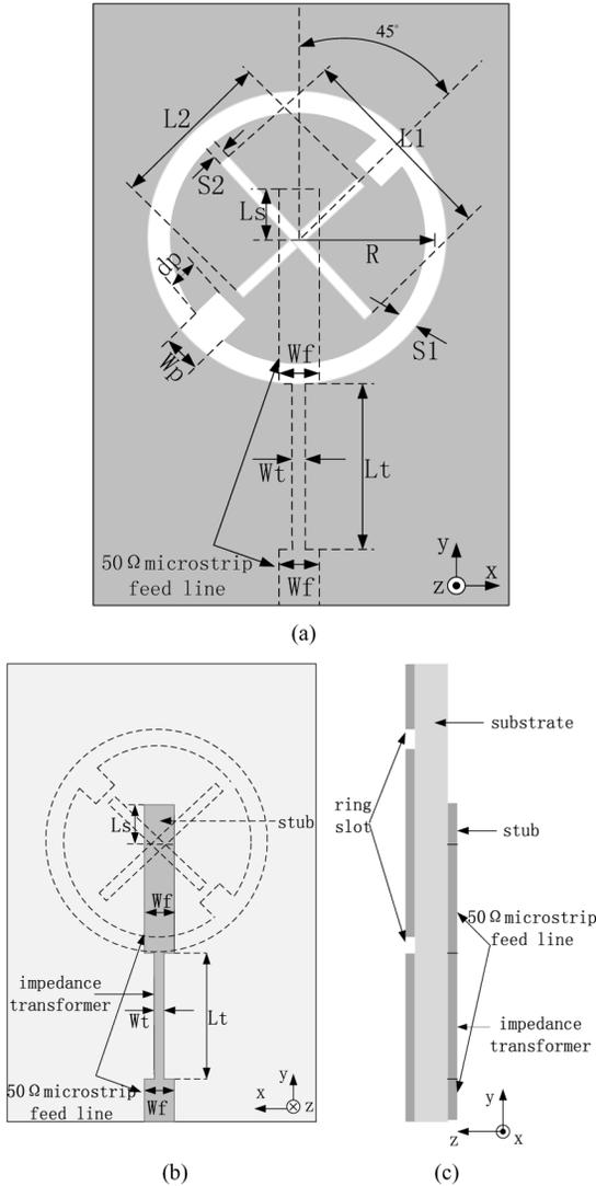
Fig. 1. Geometry of proposed dual-frequency dual CP printed slot antenna. (a) Top view. (b) Back view. (c) Side view.
