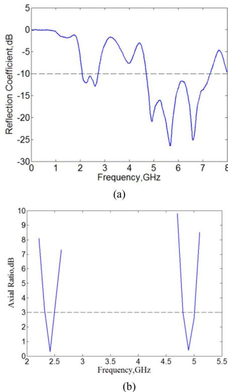
Fig. 11. Measured (a) reflection coefficient and (b) axial ratio for antenna prototype with  $\epsilon_r = 2.2$ ,  $h = 3$  mm;  $R = 16$  mm,  $d_p = 5$  mm,  $W_p = 5$  mm,  $L1 = 11$  mm,  $\Delta L = 2.5$  mm,  $S1 = S2 = 1.3$  mm;  $W_t = 3.8$  mm,  $L_t = 22$  mm, and  $L_s = -2$  mm.
