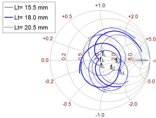
Fig. 4. Effect of various  $L_t$  on the input impedance of the antenna;  $W_t = 0.9$  mm,  $L_s = 1$  mm;  $f_L = 2.4$  GHz, and  $f_U = 5.8$  GHz.
