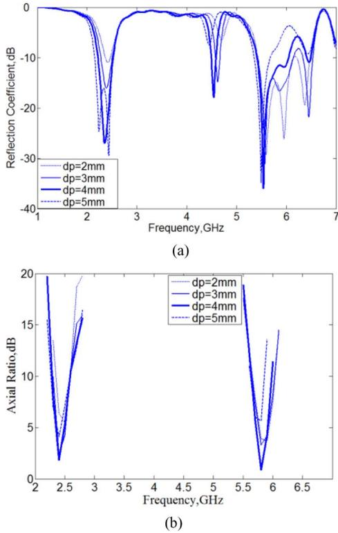
Fig. 6. Simulated (a) reflection coefficient and (b) axial ratio against frequency for various  $d_p$ .  $R = 14$  mm,  $W_p = 3$  mm,  $L1 = 8$  mm, and  $\Delta L = 1.5$  mm.
