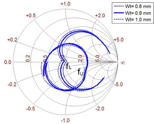
Fig. 3. Effect of various  $W_t$  on the input impedance of the antenna;  $L_t = 18$  mm,  $L_s = 1$  mm;  $f_L = 2.4$  GHz, and  $f_U = 5.8$  GHz.
