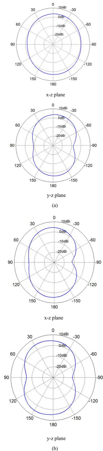
Fig. 10. Simulated radiation patterns for antenna in Fig. 9. (a)  $f = 2.5$  GHz. (b)  $f = 6.5$  GHz.
