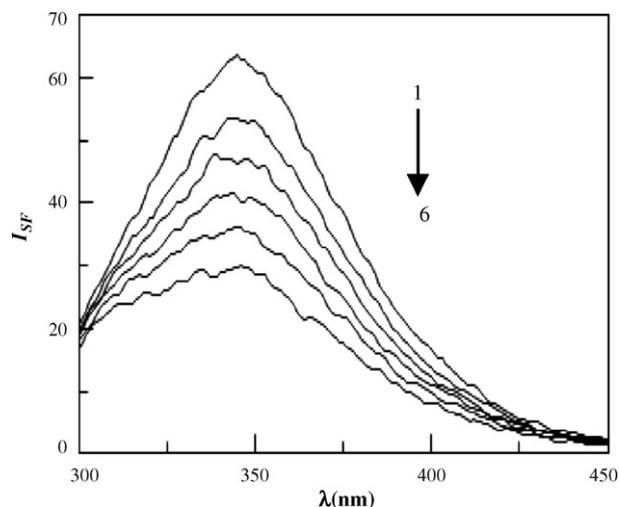
Fig. 2. The fluorescence spectra of daunorubicin–HSA system. From 1 to 6:  $C_{\text{HSA}} = 2.0 \times 10^{-5}$  M;  $C_{\text{daunorubicin}} = 0, 0.8, 1.6, 2.4, 3.2, 4.0 \times 10^{-5}$  M.
