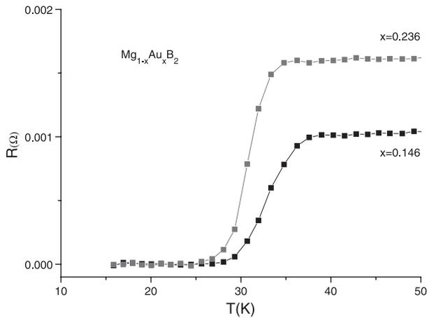
Fig. 1. Temperature dependence of the resistance of superconducting  $\text{Mg}_{1-x}\text{Au}_x\text{B}_2$  samples.
