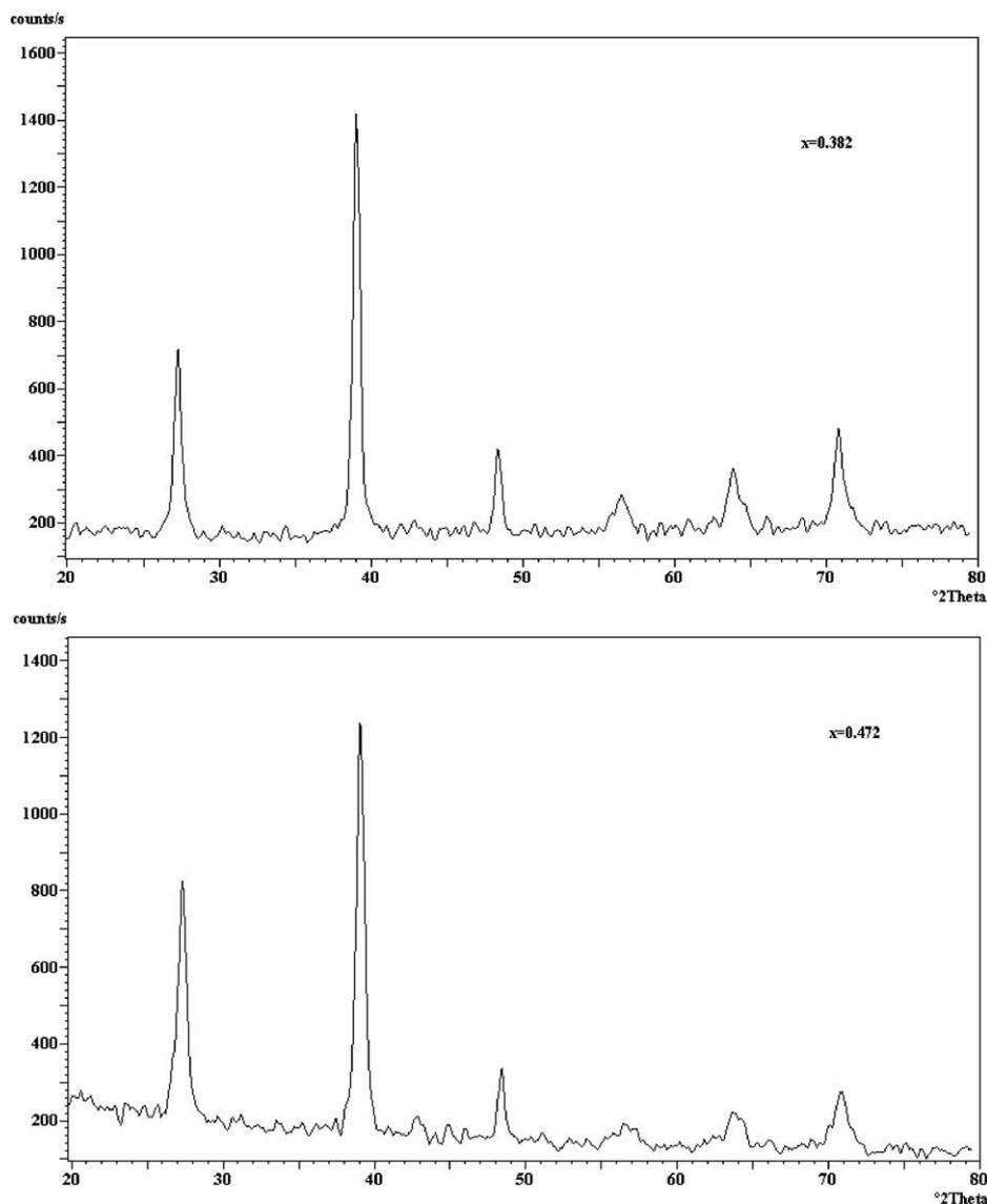
Fig. 4. XRD of  $\text{Mg}_{1-x}\text{Au}_x\text{B}_2$  with  $x=0.382$  and  $0.472$ .
