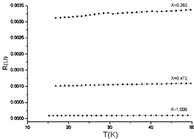
Fig. 2. Metallic  $R$ - $T$  dependence of the Au-doped  $\text{Mg}_{1-x}\text{Au}_x\text{B}_2$  with  $x \geq 0.382$ .
