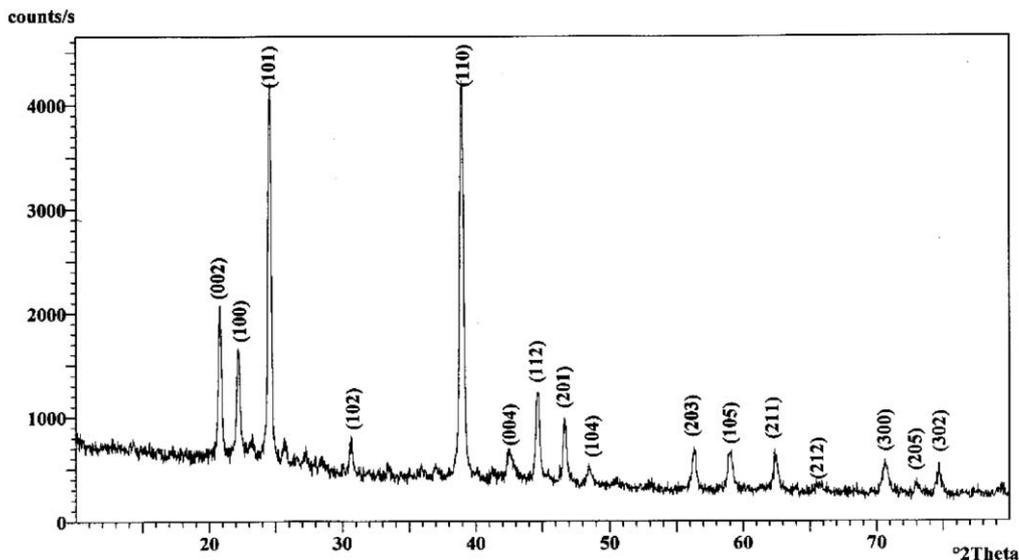
Fig. 3. Powder X-ray diffraction pattern of  $\text{Mg}_{0.854}\text{Au}_{0.146}\text{B}_2$ .
