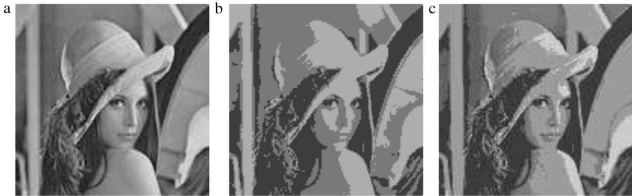
**Fig. 6.** Image segmentation worked with  $128 \times 128$  Lena image using the CLM-CNN method. (a) Original image; (b) Image segmented with 3 layers ; (c) Image segmented with 6 layers.
