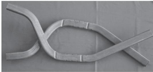
Fig. 15 Hydroformed front beam holder.
