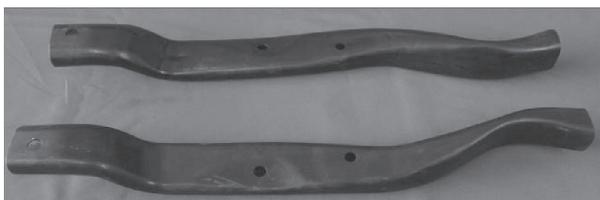
Fig. 16 Hydroformed engine cradle chassis.
