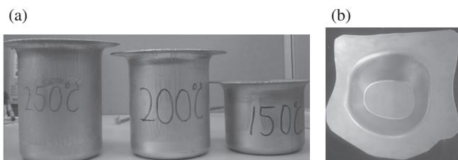
Fig. 23 Warm hydroformed part with heated oil. (a) Cups with different temperature (b) aluminum part.
