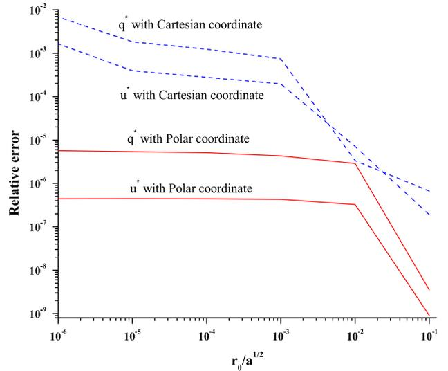
Fig. 8. Comparisons for the results at point (0.2,0.2) between the polar and Cartesian coordinate systems with kernels  $u^*$  and  $q^*$ .
