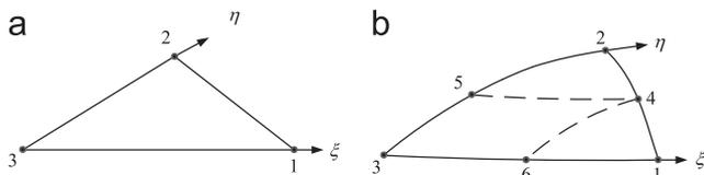
Fig. 1. Node distributions for triangular elements: (a) planar triangular element; (b) curved triangular element.
