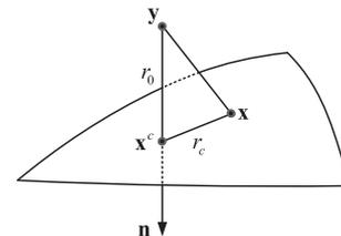
Fig. 2. The projection from the source point  $\mathbf{y}$  to the triangular element.
