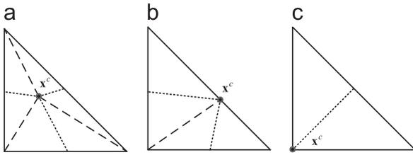
Fig. 4. Subdivision into sub-triangles when the nearly singular point is located (a) inside the element; (b) on one side; (c) on one vertex.
