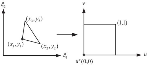
Fig. 5. Mapping each sub-triangle into a quadrangle.
