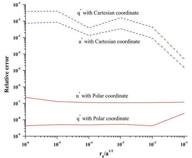
Fig. 10. Comparisons for the results at point (0.2,0.6) between the polar and Cartesian coordinate systems with kernels  $u^*$  and  $q^*$ .
