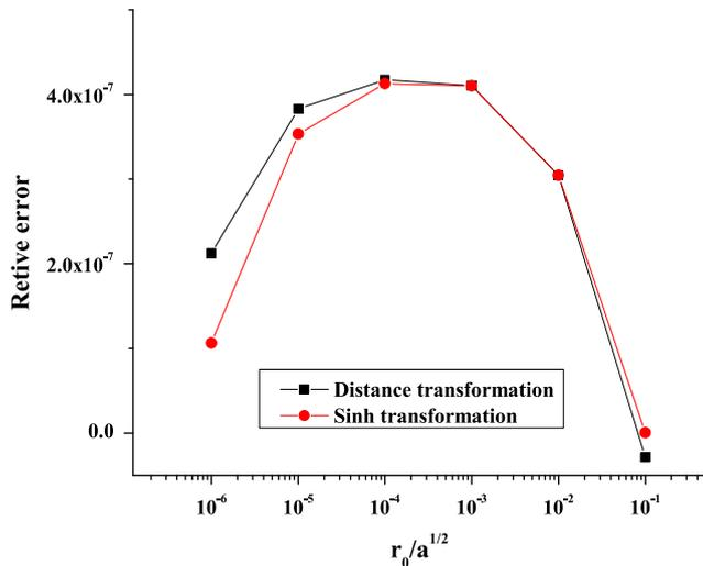
Fig. 12. Comparisons for the results at point (0.2,0.2) between the distance and sinh transformations with kernels  $u^*$ .
