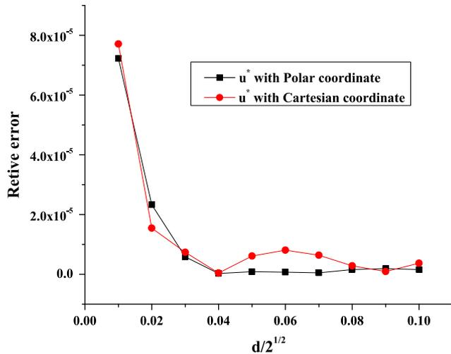
Fig. 11. Relative errors for the polar and Cartesian coordinate systems with kernel  $u^*$  corresponding to various values of  $d$ .
