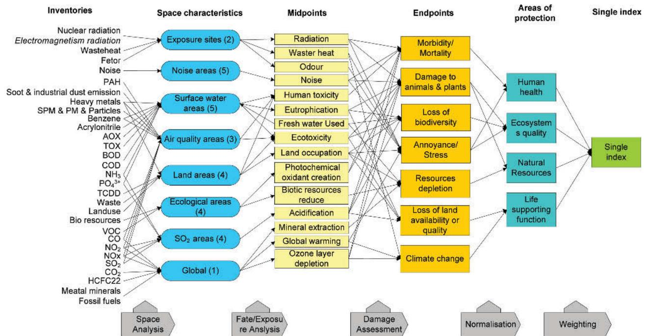
Figure 1. The framework of the LCIA method.
