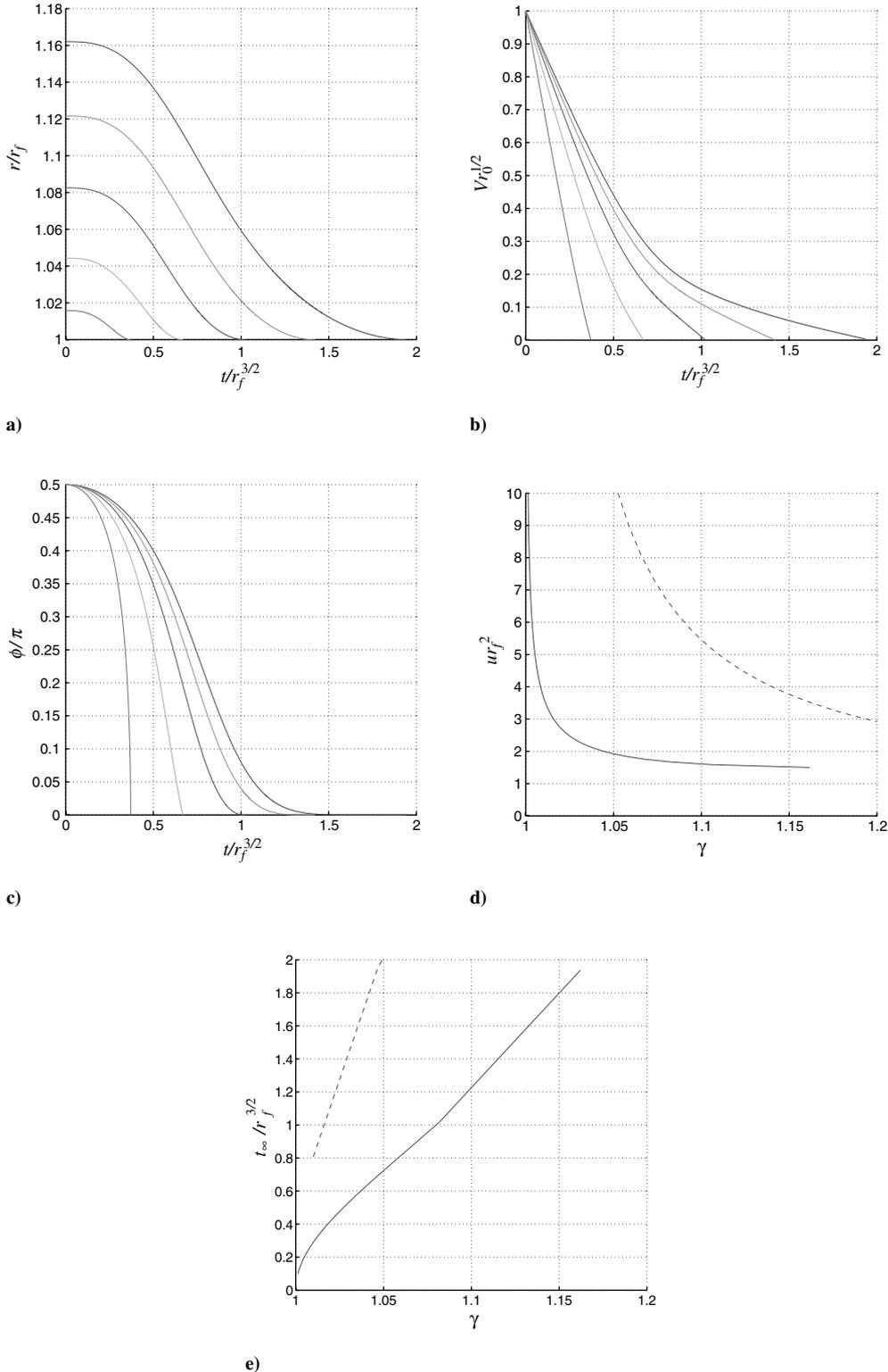
Fig. 3 The solutions:  $r(t)$ ,  $V(t)$ ,  $\phi(t)$  for  $\gamma = 1.16, 1.12, 1.08, 1.04, 1.02$ : d) required control  $ur_f^2$  and e) time of descent  $t_\infty$  are plotted as a function of  $\gamma$  together with the corresponding plots (the dotted lines) from Fig. 2. Notice that the lower values of  $\gamma$  correspond to shorter times of descent.
