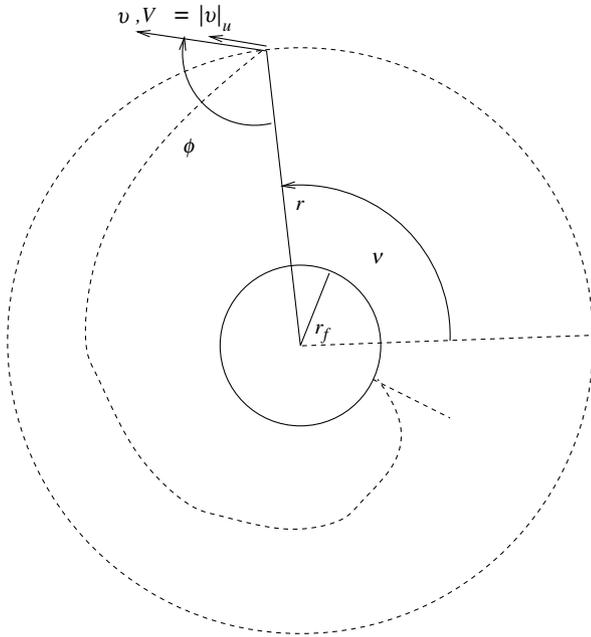
**Fig. 1** A schematic definition of the variables used in the analysis:  $(r, v)$  are polar coordinates of the satellite position  $x \in \mathbb{R}^2$ ,  $V$  is the norm of the velocity, and  $\phi$  is the angle between  $\dot{x}$  and  $x$ .
