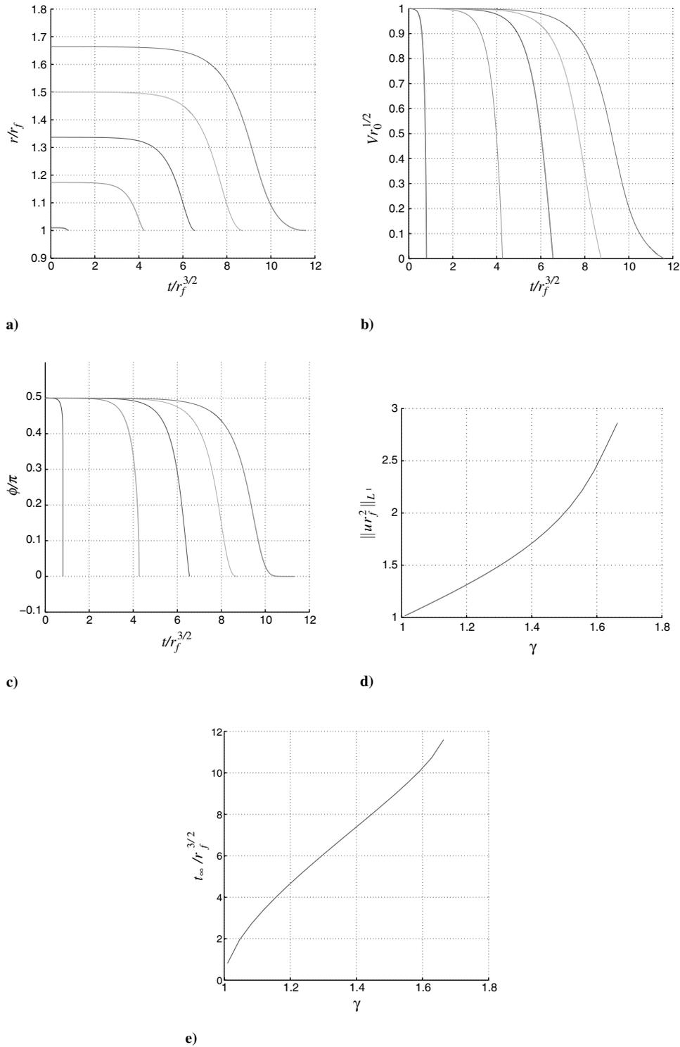
**Fig. 2** The solutions: a)  $r(t)$ , b)  $V(t)$ , and c)  $\phi(t)$  for five equidistant  $\gamma$  values between 1.01 and 1.69 for the angle-dependent controller, and d) consumed control  $\|u\|_{L^1}$  and e) time of descent  $t_\infty$  as a function of  $\gamma$ .
