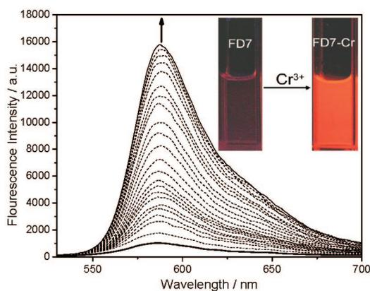
**Figure 4.** Fluorescence emission changes of **FD7** (20 μM) in ethanol/H<sub>2</sub>O (1:1, v/v, pH 7.4) solutions upon addition of Cr<sup>3+</sup> (0–45 equiv). Each spectrum was acquired 1 min after Cr<sup>3+</sup> addition,  $\lambda_{\text{ex}} = 530$  nm. Fluorescence photograph was obtained under irradiation of UV light (365 nm).
