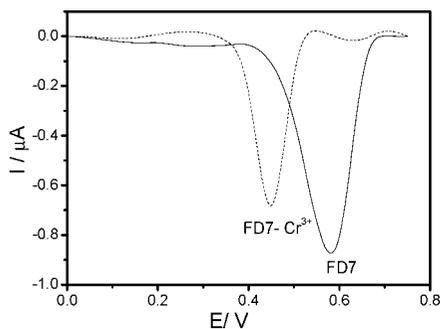
**Figure 3.** DPV of **FD7** (100 μM) in ethanol solution in the absence and presence of 1.6 equiv of Cr<sup>3+</sup> with *n*-Bu<sub>4</sub>NPF<sub>6</sub> as supporting electrolyte.
