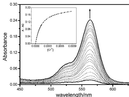
**Figure 2.** Changes in UV–vis absorption spectra of **FD7** (20  $\mu$ M) in ethanol/H<sub>2</sub>O (1:1, v/v, pH 7.4) solutions with various amounts of Cr<sup>3+</sup> ions (0–45 equiv). Inset: Absorbance at 565 nm of **FD7** as a function of Cr<sup>3+</sup> concentration.
