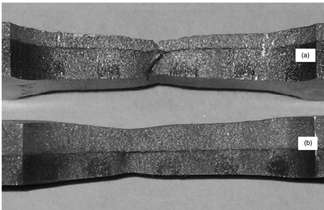
**Fig. 8** Macrographs of interface fracture (a) fracture side of stainless steel and (b) interface detachment
