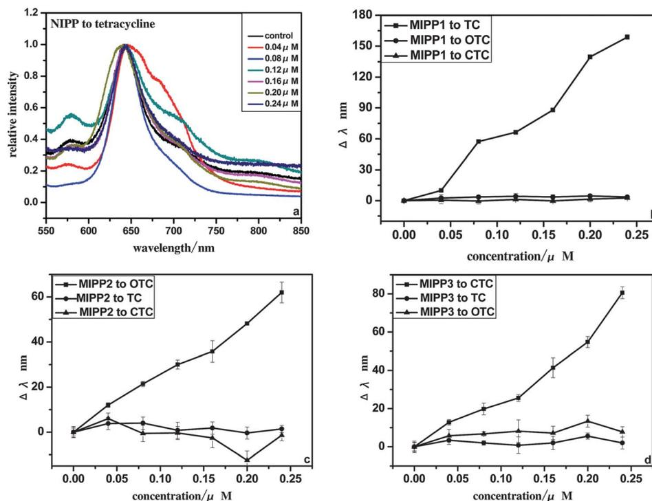
**Fig. 6** (a) Response of NIPP to TC and response of MIPP1 (b), MIPP2 (c), and MIPP3 (d) to TC, OTC and CTC in the same variation of concentrations.
