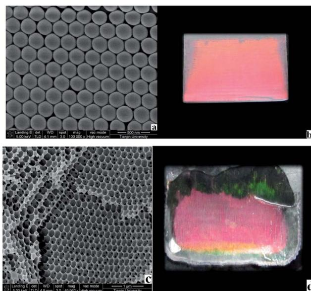
**Fig. 3** Typical SEM image (a) and photograph (b) of the used PS colloidal crystal template, and typical SEM image (c) and photograph (d) of the resulting MIPP film.
