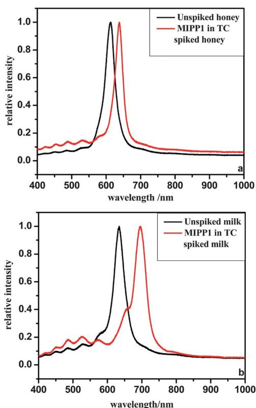
**Fig. 8** Diffraction response of MIPPI in the TC spiked honey (a) and milk (b) sample.
