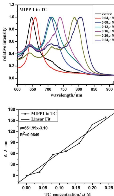
**Fig. 4** (a) Diffraction response of MIPP1 to TC solution of varying concentrations. (b) Relationship between the  $\Delta\lambda$  of diffraction peak and the concentration of TC in the range from 0.04  $\mu\text{M}$  to 0.24  $\mu\text{M}$ .
