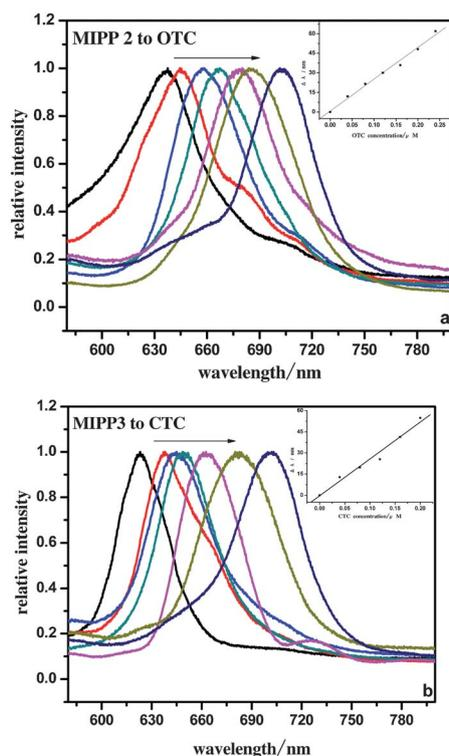
**Fig. 5** (a) Diffraction response of MIPP2 to OTC and (b) MIPP3 to CTC solutions of varying concentrations. The inset is the fit relationship between the  $\Delta\lambda$  of the diffraction peak and the concentration of TCs in the range from 0.04  $\mu\text{M}$  to 0.24  $\mu\text{M}$ .
