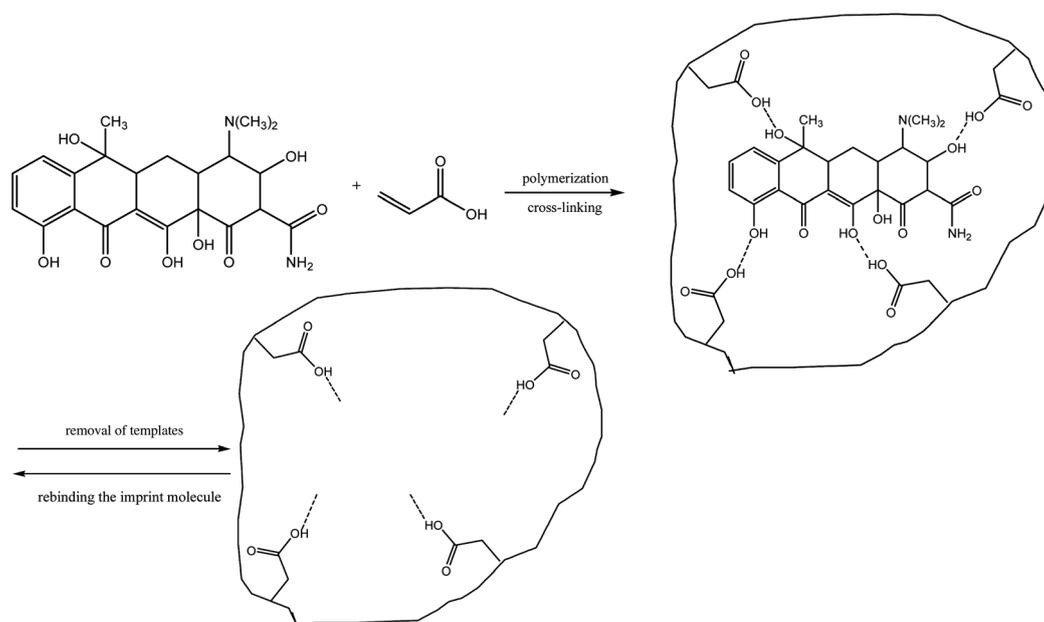
**Fig. 7** The establishment and interruption process of the hydrogen bonding between the functional monomer AA and the TC template molecule.
