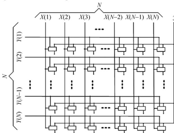
Figure 9 The array driving circuits used for the SPR display with  $N \times N$  pixels.
