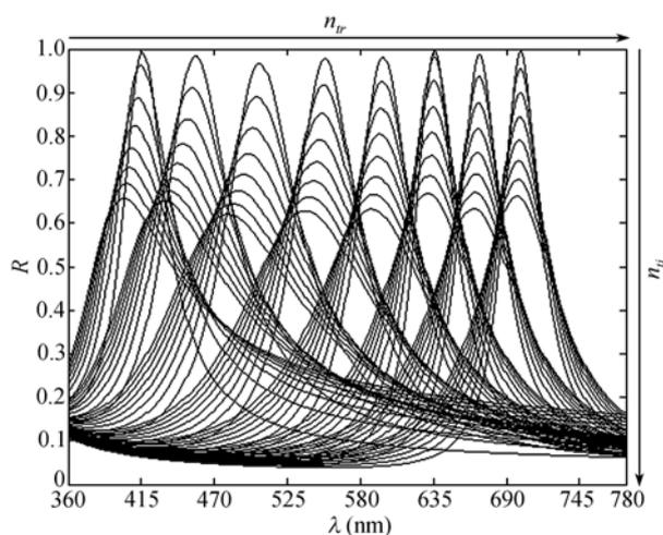
**Figure 5** The relationship of the layer 4  $n_{tr}$  and  $\lambda$ , and the relationship of the layer 6  $n_{ti}$  and  $R_{\min}$  based on the configuration of Figure 4.
