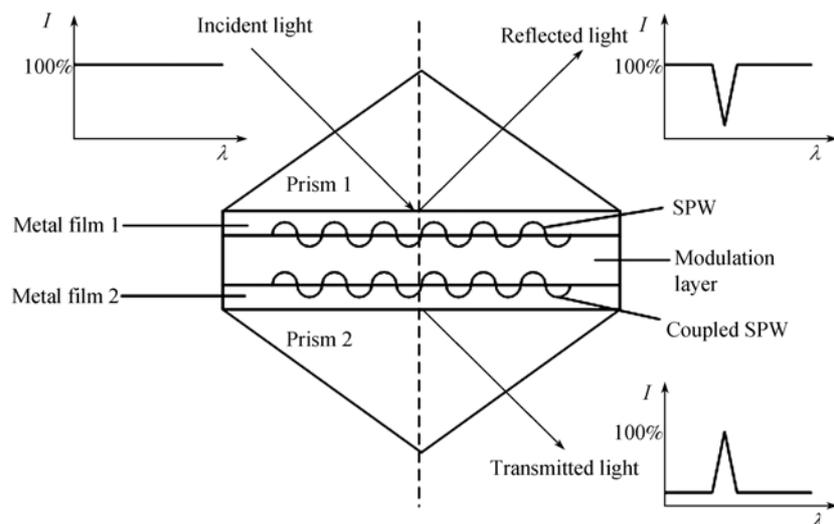
Figure 1 Basic SPR display pixel configuration.
