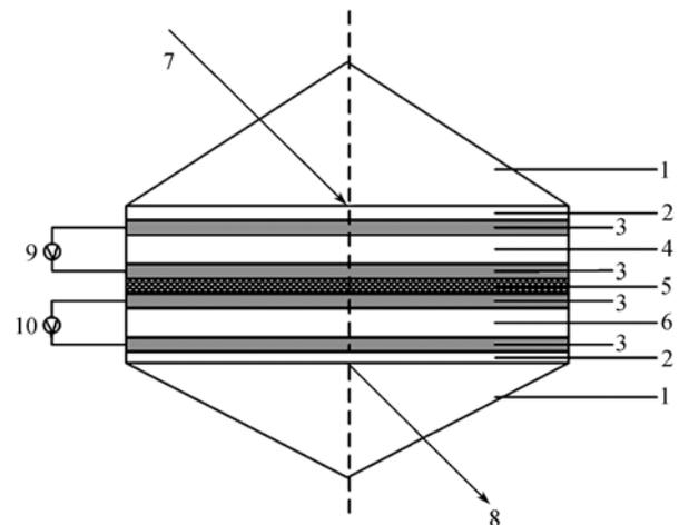
Figure 4 Combined SPR display pixel configuration. 1, Prism; 2, transition layer; 3, metal films (i.e. electric poles); 4, modulation layer with a controllable refractive index real part; 5, insulation layer; 6, modulation layer with a controllable refractive index imaginary part; 7, incident light; 8, transmitted light; 9, electrical signal to control layer 4; 10, electrical signal to control layer 6.
