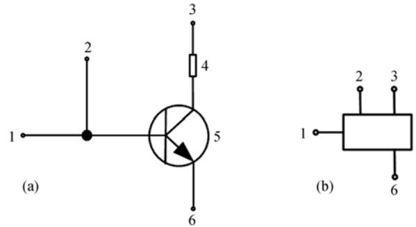
Figure 10 Driving circuit used for an SPR display pixel. (a) Circuit; (b) simplified denotation. 1, Line scan signal; 2, row scan signal; 3, color or brightness control signal; 4, load; 5, control gate; 6, loading electrical pole.
