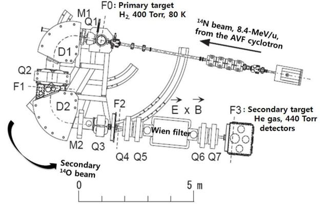
Fig. 1. Schematic view of the RI beam separator of CRIB [7]. This CRIB is composed of two parts, a double achromatic focal system (Q1, M1, D1, Q2, D2, M2, and Q3) and the Wien filter (Q4, Q5, and  $\vec{E} \times \vec{B}$ ).
