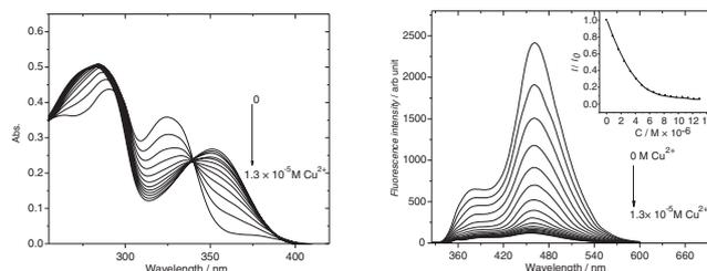
**Figure 1.** (left) Variation of the absorption spectra of **1** ( $1 \times 10^{-5} \text{ mol dm}^{-3}$ ) in water with increasing concentrations of copper(II) ions (0–13  $\mu\text{M}$ ). (right) Fluorescence emission spectra of **1** ( $1 \times 10^{-5} \text{ mol dm}^{-3}$ ) in water with increasing concentrations of copper(II) ions excited at 320 nm. (inset) Fluorescence emission plotted as a function of concentrations of copper(II) ions (0–13  $\mu\text{M}$ ).
