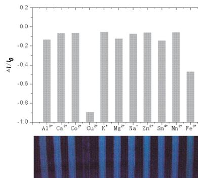
**Figure 2.** The selectivity of compound **1** to various metal ions. Concentration of compound **1** in water is  $1 \times 10^{-5} \text{ mol dm}^{-3}$ . Concentrations of all the metal ions are  $5 \times 10^{-4} \text{ mol dm}^{-3}$ .
