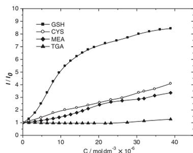
**Figure 4.** The dependence of the relative fluorescent intensity of compound **1** ( $1 \times 10^{-5} \text{ mol dm}^{-3}$ ) and copper(II) ions ( $1.3 \times 10^{-5} \text{ mol dm}^{-3}$ ) on the different sulfhydryl compounds at various concentrations in pure water. GSH (■); CYS (○); MEA (□); TGA (▲).
