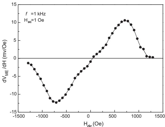
**Fig. 5.** ME voltage coefficient  $dV_{ME}/dH$  as a function of DC magnetic bias  $H_{dc}$  for Fe-Ga/BTO laminate.
