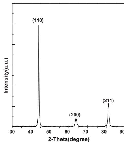
**Fig. 2.** X-ray diffraction result of Fe–Ga rod.
