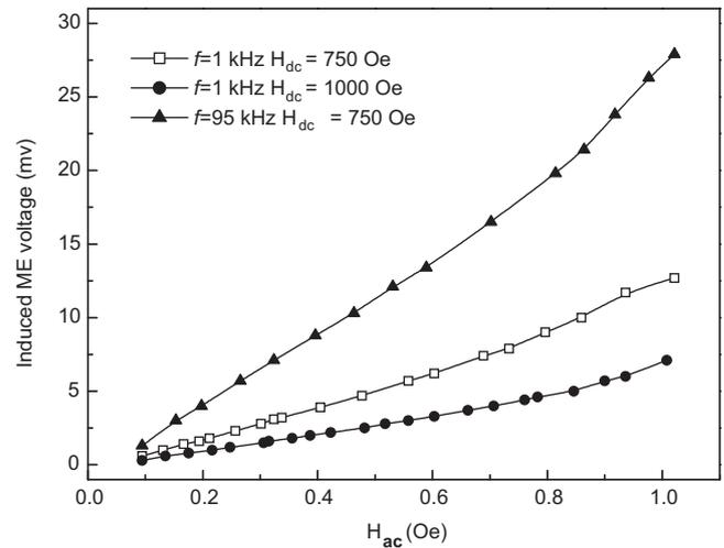
**Fig. 6.** Induced ME voltages as a function of AC magnetic field  $H_{ac}$  for Fe-Ga/BTO laminate, taken at various DC magnetic biases. The operate frequency of  $H_{ac}$  is low frequency (1 kHz) or resonance frequency (95 kHz).
