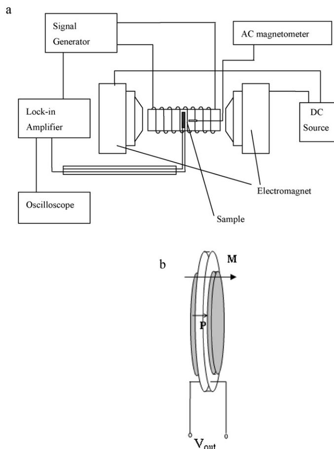
**Fig. 1.** (a) Schematic diagram of magnetolectric measurement setup and (b) illustration of the ME laminate composite.
