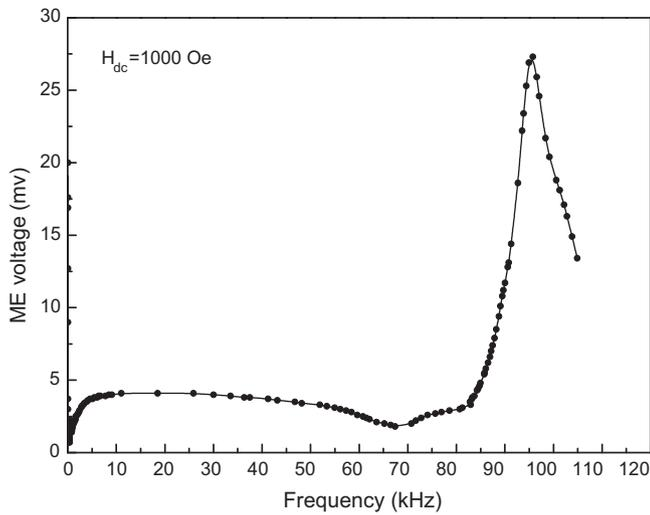
**Fig. 4.** Induced ME voltage as a function of AC magnetic field frequency for Fe-Ga/BTO laminate. These data were taken under a constant DC magnetic bias ( $H_{dc} = 1000$  Oe) and the amplitude of AC magnetic field  $H_{ac} = 1$  Oe.
