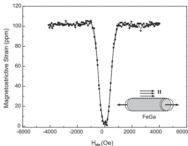
**Fig. 3.** Magnetostrictive strains of Fe–Ga rod. Inset illustrates the induced shape change of the specimen.
