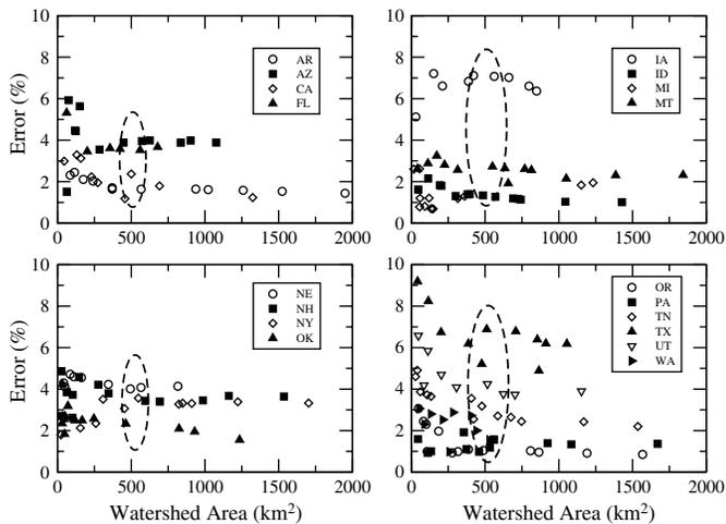
**Fig. 10.** Scatter plots of errors in downscaled TIDs versus watershed area; ellipses indicate where errors appear to reach a minimum
