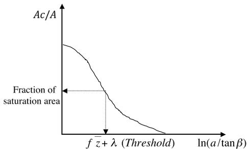
**Fig. 1.** Schematic plot of the fraction of the saturation area ( $A_c/A$ ) versus the topographic index  $\ln(a/\tan\beta)$ , which is also the complementary distribution of the topographic index; the saturation area can be determined by the interception of the threshold  $f\bar{z} + \lambda$  and the curve of  $A_c/A$  versus  $\ln(a/\tan\beta)$
