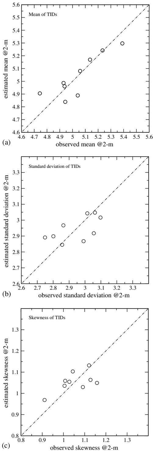
**Fig. 4.** Scatterplots of the estimated and the observed: (a) mean; (b) standard deviation; (c) coefficient of skewness of TIDs of nine catchments over Oak Ridge Reservation; the observed moments of TIDs are directly computed on the basis of 2-m TIDs, and the estimated moments are computed from downsampled TIDs from 10 to 2 m
