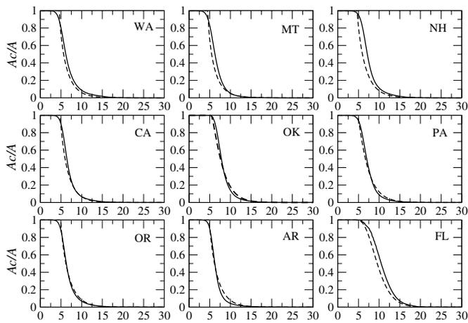
**Fig. 9.** Plots of TIDs of nine major watersheds in nine states observed at 10 m (solid) and downscaled from 1 km to 10 m through correcting three moments (dashed)
