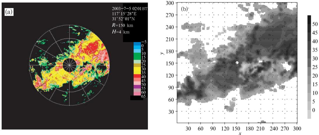
**Fig.1.** Comparison of 4-km height reflectivities (dBz) between (a) CAPPI image (range 150 km, Hefei radar, 0201 BT 5 July 2003) and (b) output treated by this paper's technique (grid spacing 1 km) at Hefei.
