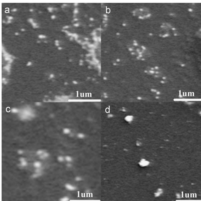
Fig. 5. FESEM images showing distribution of  $\text{LaB}_6$  particles in PMMA matrix. (a), (b), (c) and (d), respectively, depict distribution of particles with sizes of 50 nm, 70 nm, 150 nm and 400 nm.
