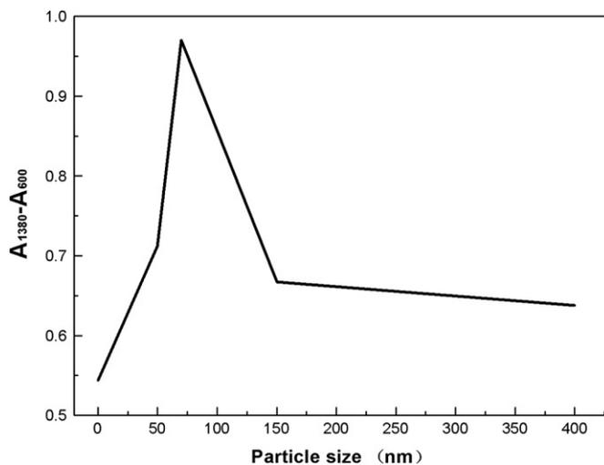
Fig. 7. Relative strength of light absorption concerning composites containing  $\text{LaB}_6$  particles in different sizes. 0 nm stood for pure polymer without  $\text{LaB}_6$  particles.
