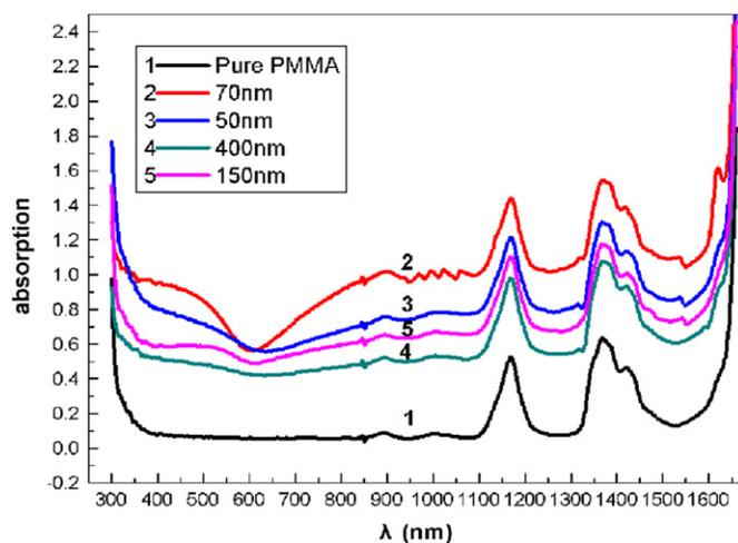
Fig. 6. Absorption spectrum of  $\text{LaB}_6/\text{PMMA}$  composites from 300 nm to 1600 nm.
