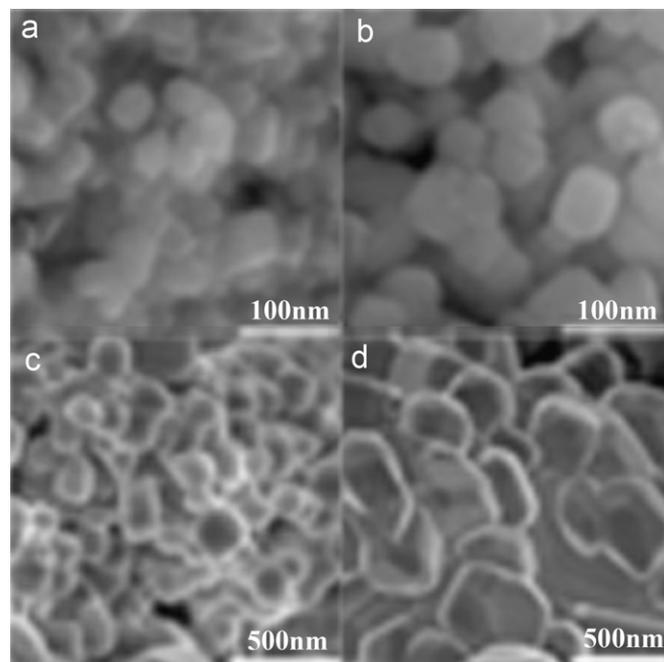
**Fig. 3.** FESEM images of  $\text{LaB}_6$  particles in different sizes. (a), (b), (c) and (d) show particles with size of 50 nm, 70 nm, 150 nm and 400 nm, respectively.
