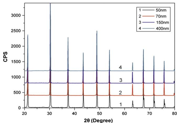
**Fig. 2.** XRD results of  $\text{LaB}_6$  particles in different sizes.
