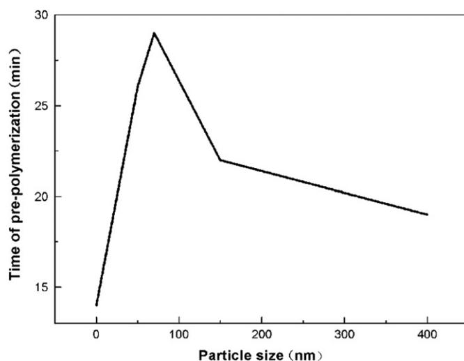
**Fig. 4.** Size effect on time needed for pre-polymerization of MMA. 0 nm stood for pure MMA without  $\text{LaB}_6$  particles.
