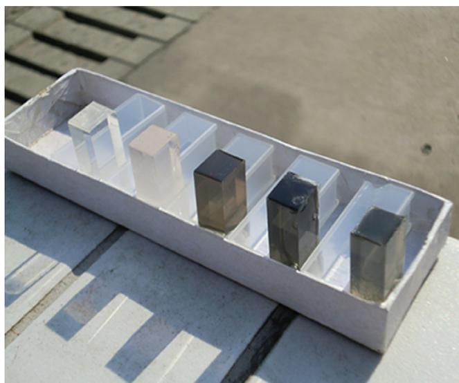
**Fig. 1.** Molds and final composites' samples. The left sample was made of pure MMA without  $\text{LaB}_6$  added in; the others were made of mixture of MMA and  $\text{LaB}_6$  particles.
