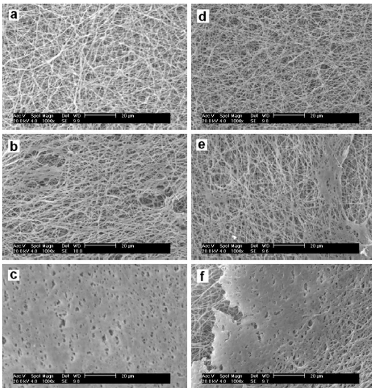
**Figure 6** SEM micrographs of electrospun PLLA/BTEAC membranes after degradation: (a) dynamic condition 2 h, (b) dynamic condition 6 h, (c) dynamic condition 10 h, (d) static condition 2 h, (e) static condition 6 h, and (f) static condition 10 h.
