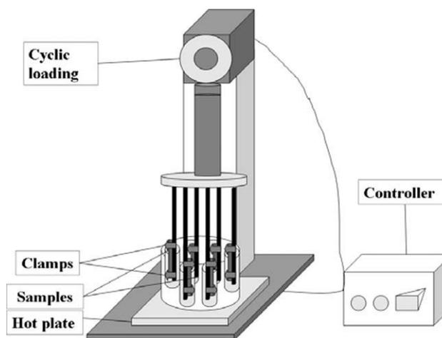
Figure 1 Cyclic stretch apparatus for degradation.
