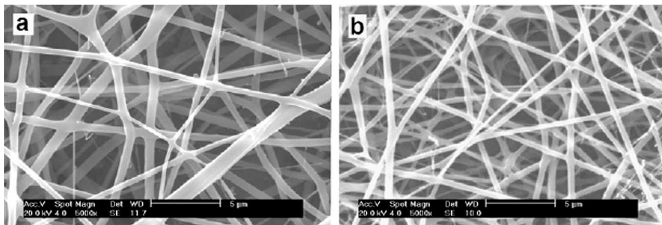
**Figure 2** SEM micrographs of electrospun membranes: (a) PLLA, (b) PLLA/BTEAC.
