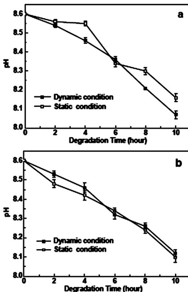
Figure 4 Variations of pH for buffer solution during degradation of electrospun membranes: (a) PLLA, (b) PLLA/BTEAC.
