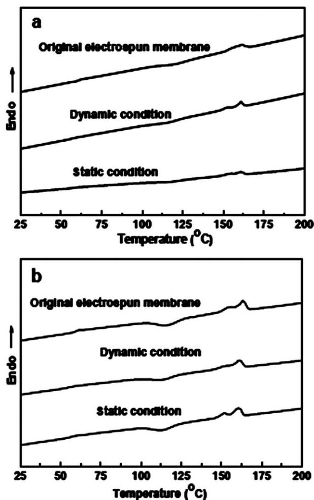
Figure 7 DSC traces for original electrospun membranes and specimens after degradation for 10 h: (a) PLLA, (b) PLLA/BTEAC.
