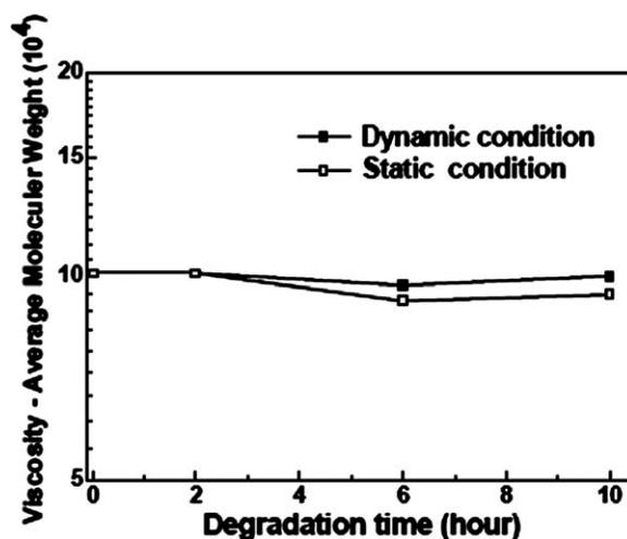
Figure 8 Viscosity-average molecular weight of PLLA during degradation.
