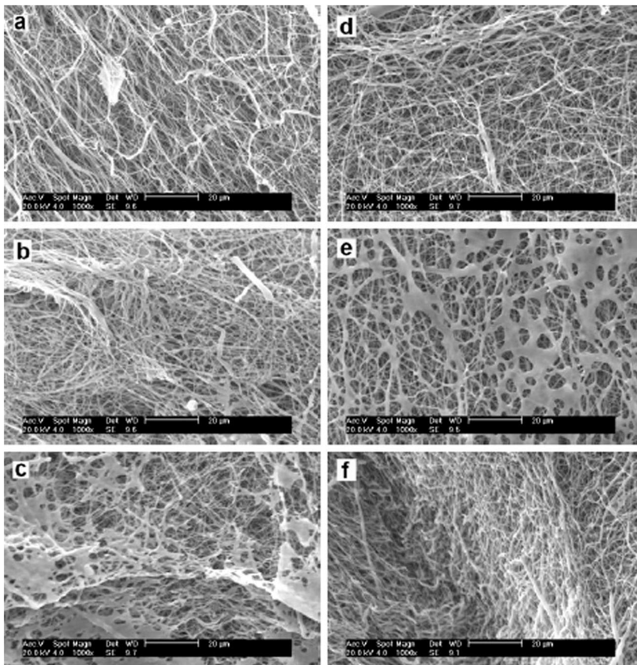
**Figure 5** SEM micrographs of electrospun PLLA membranes after degradation: (a) dynamic condition 2 h, (b) dynamic condition 6 h, (c) dynamic condition 10 h, (d) static condition 2 h, (e) static condition 6 h, and (f) static condition 10 h.
