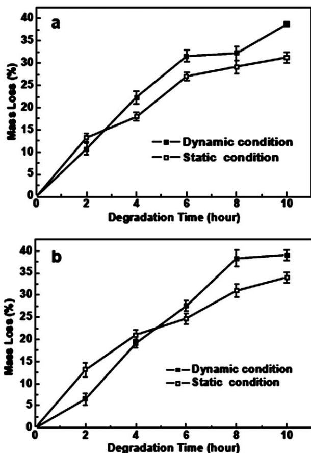
Figure 3 Mass loss of electrospun membranes during degradation: (a) PLLA, (b) PLLA/BTEAC.
