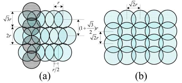
Fig. 8. Two common placements: (a) Kar's deployment pattern, (b) Square deployment pattern.
