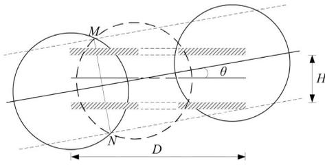
Fig. 5. Using one  $(d, r)$ -strip to cover a long belt area.
