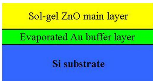
**Figure 1.** Schematic diagram of ZnO/Au/Si thin films.
