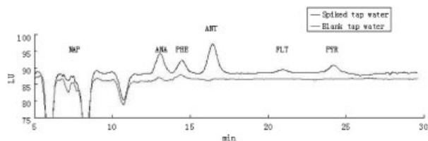
**Figure 5.** HPLC-FLD chromatograms of tap water sample obtained by continuous flow PDMS/ $\beta$ -CD/DVB-coated SPSE. Spiking concentration for all target compounds is 25 ng/L.
