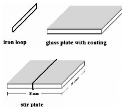
Figure 1. Setup of stir plate.
