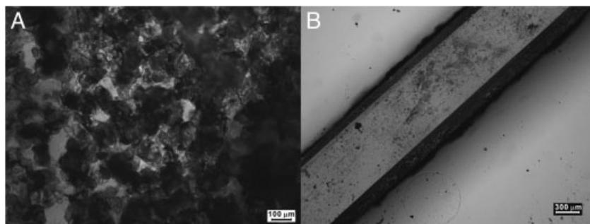
**Figure 3.** Microscope graphs of (A) the surface and (B) the cross section of PDMS/ $\beta$ -CD/DVB-coated stir plate.
