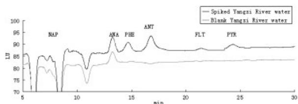
**Figure 6.** HPLC-FLD chromatograms of Yangzi River water sample obtained by continuous flow PDMS/ $\beta$ -CD/DVB-coated SPSE. Spiking concentration for all target compounds is 50 ng/L.
