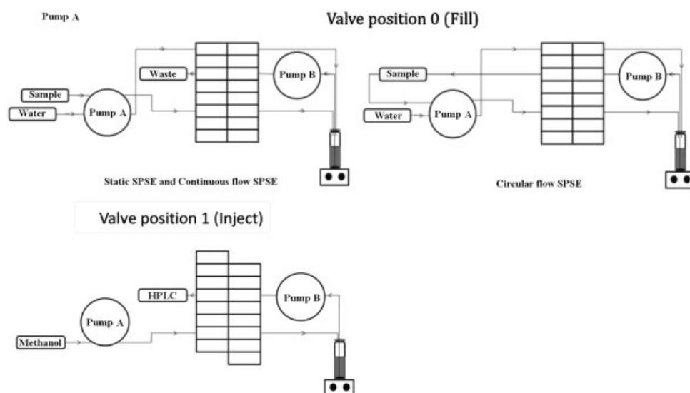
**Figure 2.** Schematic representation of static SPSE, circular flow SPSE and continuous flow SPSE.
