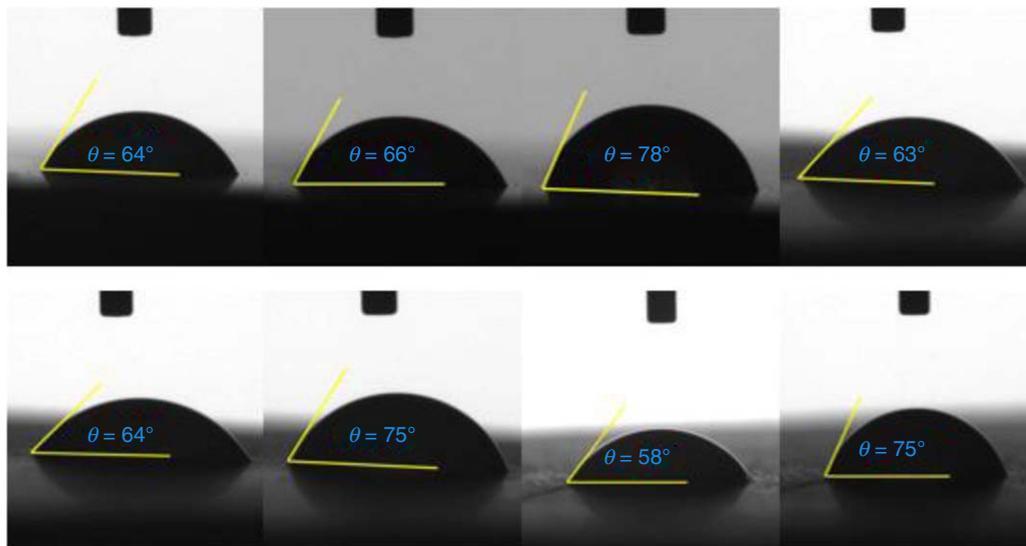
Fig. 4—Water contact angle on Montney core sample shows it is water-wet.
