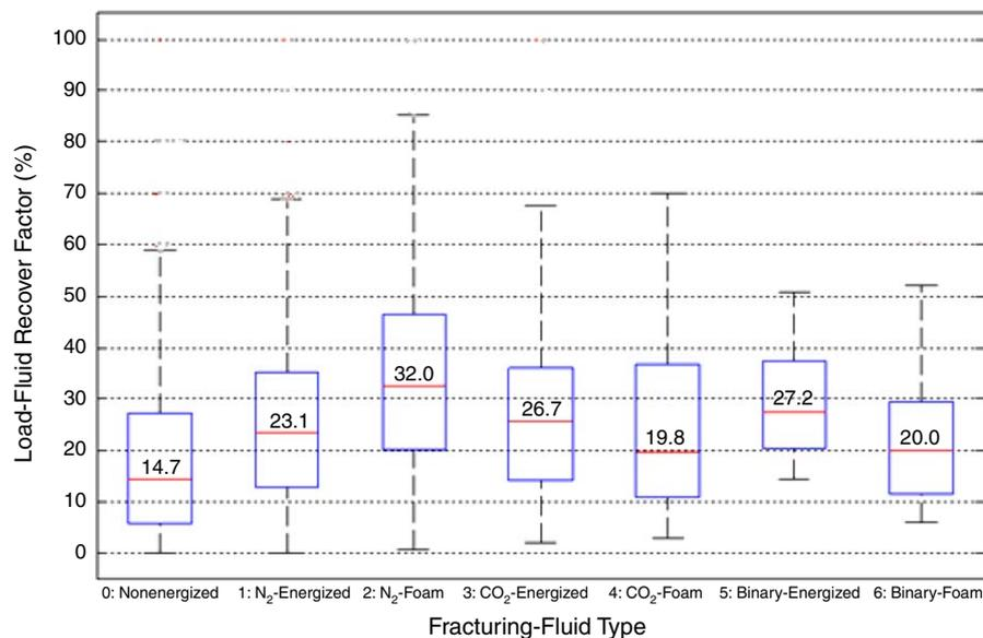
**Fig. 7—Load fluid-recovery factor for different water-based fracturing fluid in Montney (Data provided by the Canadian Discovery Ltd.'s Well Completions and Frac Database).**
