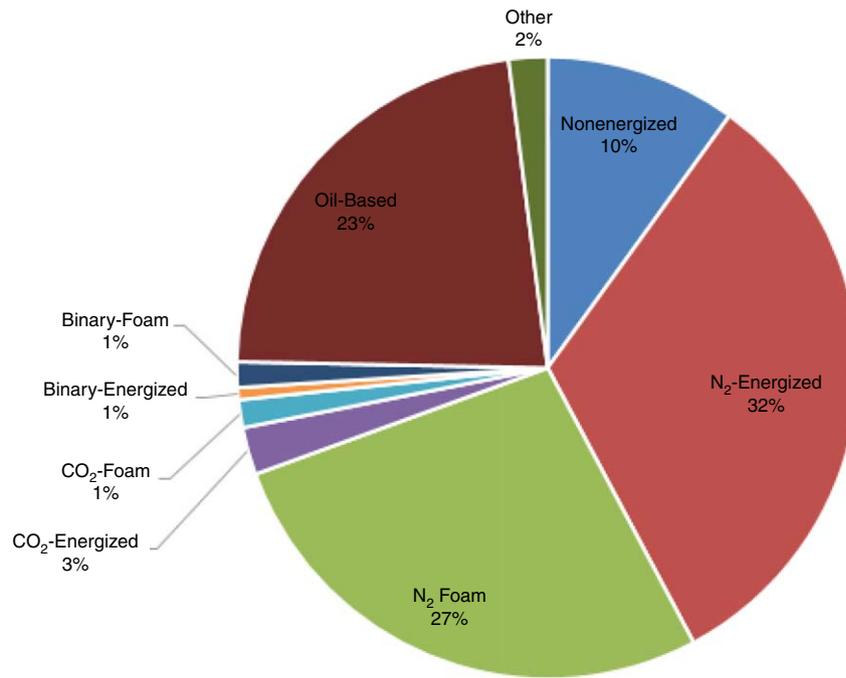
Fig. 5—Fracturing-fluid-type percentage in Montney on the basis of the data of 5,826 wells from 1975 to 2015 (Data provided by the Canadian Discovery Ltd.'s Well Completions and Frac Database).
