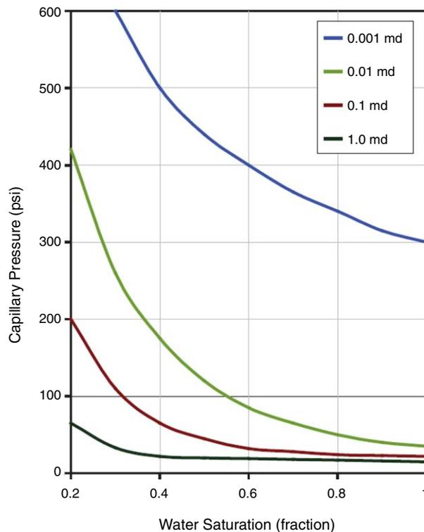
**Fig. 2—Effect of capillarity on water saturation (Economides and Martin 2007).**
