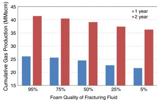
**Fig. 14—Impact of foam quality of fracturing fluid on initial production rate.**
