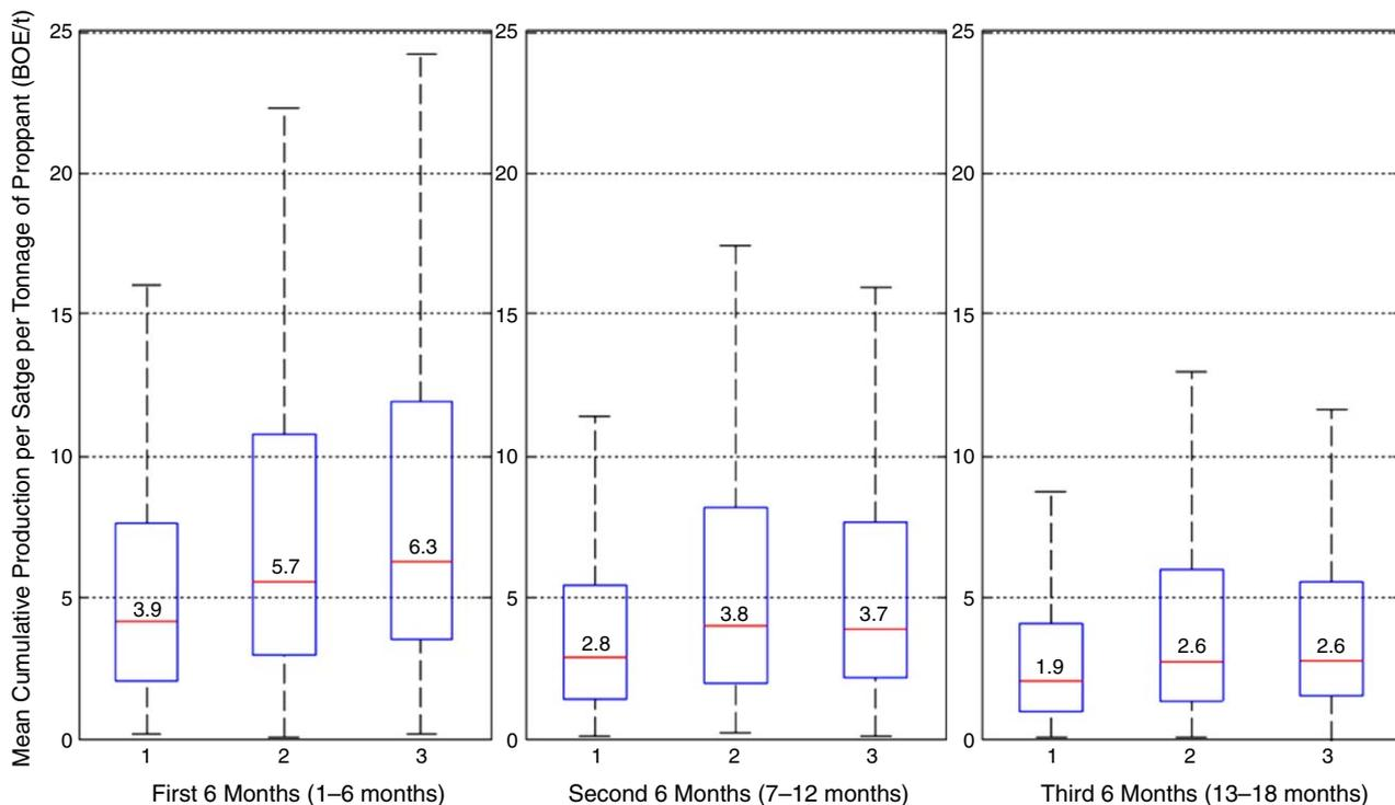
**Fig. 8—Impact of aqueous-load fluid-recovery factor on well production, 1-low-load fluid recovery < 10%; 2-medium-load fluid recovery 10 to 40%; and 3-high-load fluid recovery > 40% (Data provided by the Canadian Discovery Ltd.'s Well Completions and Frac Database).**
