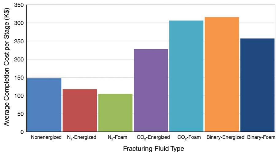
Fig. 6—Average completion cost per stage of water-based fracturing in Montney (Data provided by the Canadian Discovery Ltd.'s Well Completions and Frac Database).
