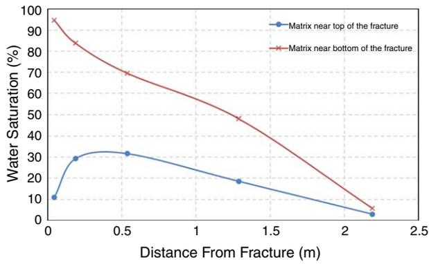
**Fig. 11—History matching of a typical N<sub>2</sub>-energized fractured well in Montney.**
