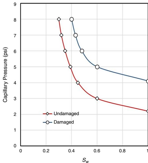
**Fig. 1—Effect of damage on the capillary pressure function (Holditch 1979).**
