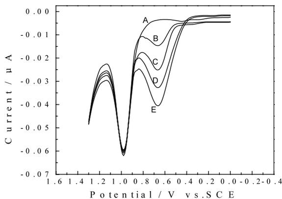
Fig. 4. Differential pulse voltammetry of  $2.0 \times 10^{-6}$  mol l $^{-1}$  procaine hydrochloride in the presence of urine acid. (A) Procaine hydrochloride; Urine acid concentration: (B)  $2.0 \times 10^{-5}$  mol l $^{-1}$ , (C)  $6.0 \times 10^{-5}$  mol l $^{-1}$ , (D)  $8.0 \times 10^{-5}$  mol l $^{-1}$ , (E)  $1.0 \times 10^{-4}$  mol l $^{-1}$ .
