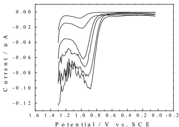
Fig. 2. Differential pulse voltammograms of  $2.0 \times 10^{-6}$  mol  $l^{-1}$  procaine hydrochloride with various contents of pumice in carbon paste electrode in phosphate buffer. The descending order of currents are 22, 15, 9, 6, 3 and 0% (m/m) of pumice in carbon paste electrode, respectively.
