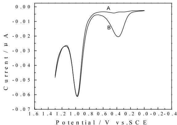
Fig. 6. Differential pulse voltammetry of  $2.0 \times 10^{-6}$  mol l $^{-1}$  procaine hydrochloride in the presence of adrenaline. (A) Procaine hydrochloride; (B)  $2.0 \times 10^{-5}$  mol l $^{-1}$  Adrenaline.
