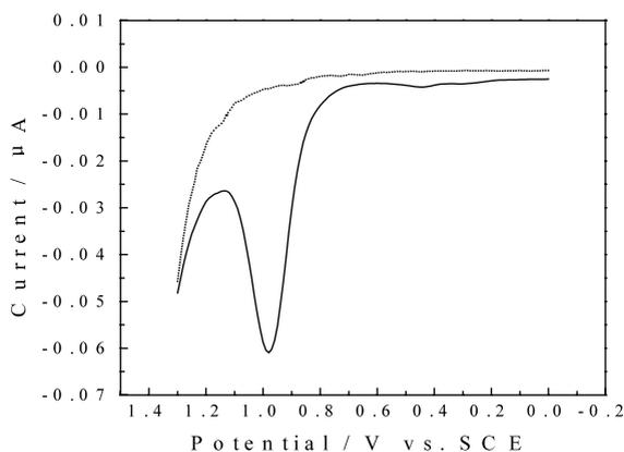
Fig. 1. Differential pulse voltammograms of the pumice carbon paste electrodes in phosphate buffer. Accumulation potential under stirring: 0.0 V, Accumulation time: 30 s, Quiet time: 20 s, pulse height: 0.050 V, sampling width: 0.05 s, pulse period: 0.2 s, sensitivity:  $1.0 \times 10^{-7}$  A/V. Solid line: in  $2.0 \times 10^{-6}$  mol l<sup>-1</sup> procaine hydrochloride. Short dot line: in absent of procaine hydrochloride.
