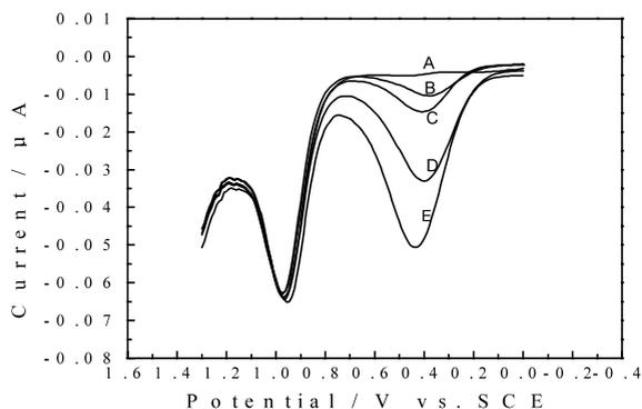
Fig. 5. Differential pulse voltammetry of  $2.0 \times 10^{-6}$  mol l $^{-1}$  procaine hydrochloride in the presence of dopamine (A) Procaine hydrochloride; Dopamine concentration: (B)  $2.0 \times 10^{-6}$  mol l $^{-1}$ , (C)  $5.0 \times 10^{-6}$  mol l $^{-1}$ , (D)  $1.0 \times 10^{-5}$  mol l $^{-1}$ , (E)  $2.0 \times 10^{-5}$  mol l $^{-1}$ .
