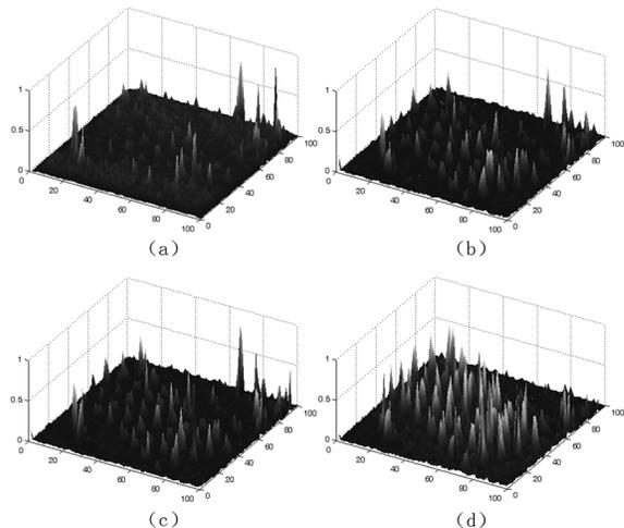
Figure 2. 3-D plot of detection results using (a) RX on original HSI, and RX after feature extraction by (b) ICA, (c) SKPCA, (d) KICA, respectively
