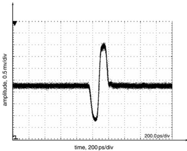
Fig. 5 Generated monocycle pulse with negative polarity
