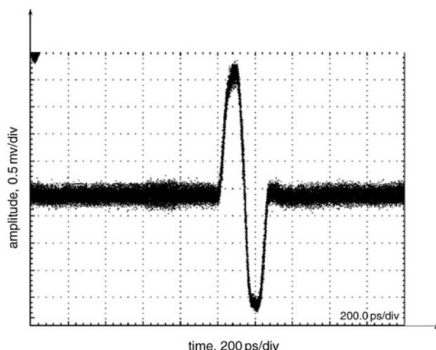
Fig. 4 Generated monocycle pulse with positive polarity
