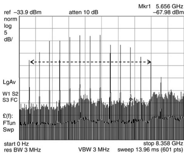
Fig. 6 Spectrum of generated monocycle pulse
