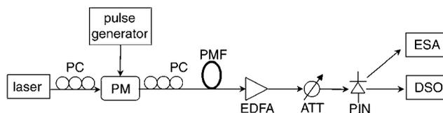
Fig. 2 Experimental setup
