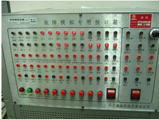
Fig. 8. Interface matrix device for fault simulation and injection.
